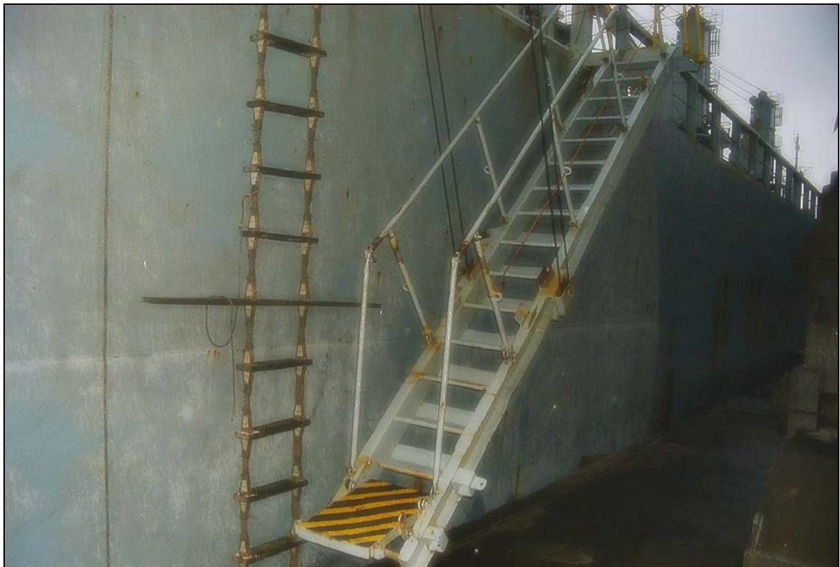
Figure 4: Subsequent demonstration of the mixed pilot ladder
