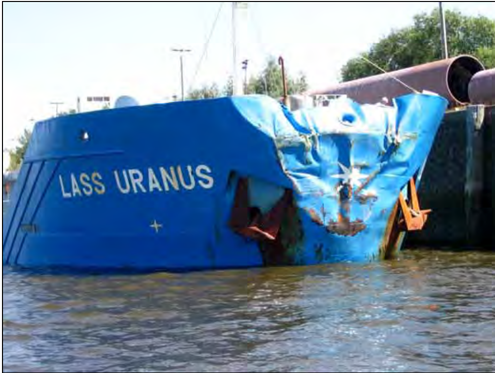
Figure 12: Damage to the LASS URANUS' stem
