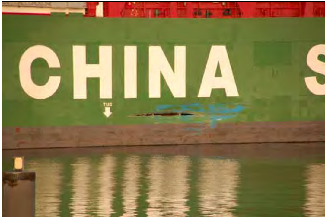
Figure 16: Close-up of the tear on the starboard side of the XIN FU ZHOU
