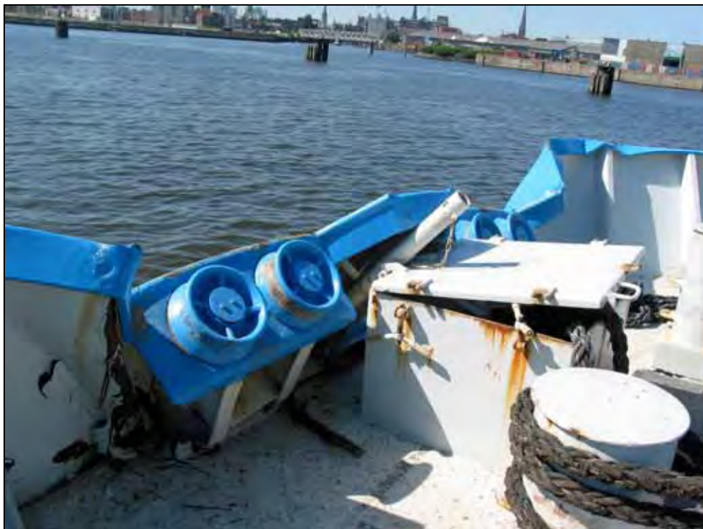
Figure 13: Damage to the forecabin of the LASS URANUS
