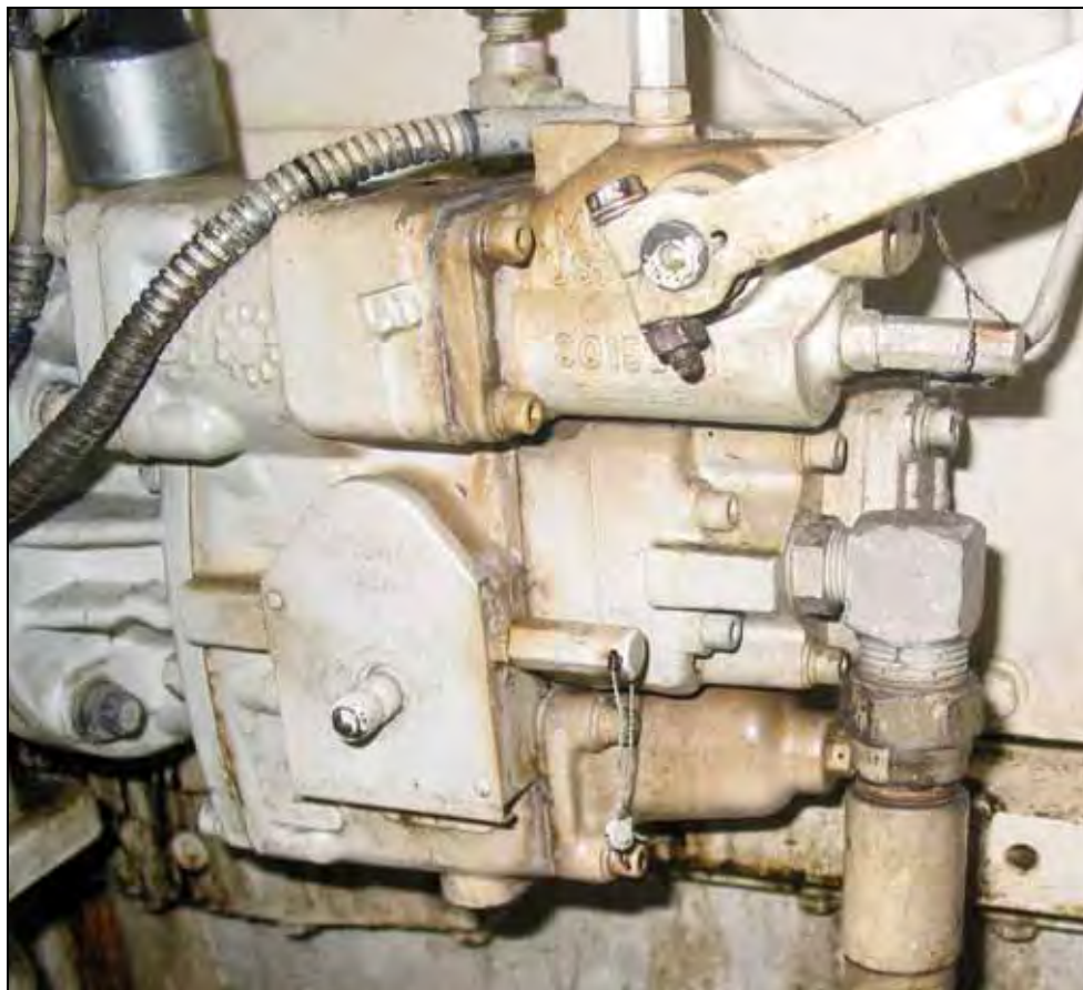
Figure 19: Leaded injection pump of the port main engine of LASS URANUS
