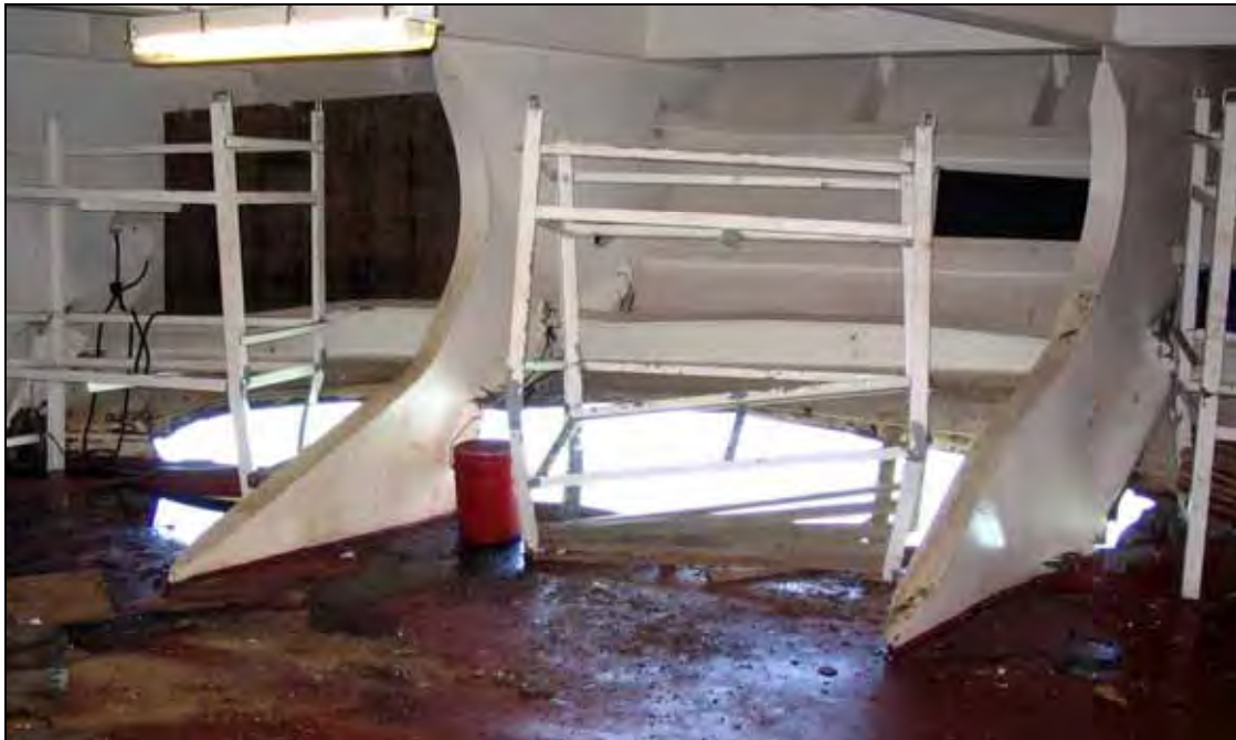
Figure 17: Tear in the hull of the HANJIN GOTHENBURG on 21 September 2007
