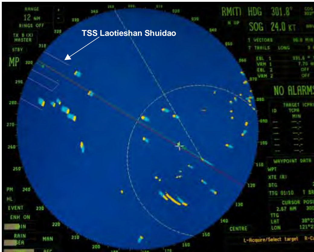
Figure 6: Radar image of the traffic volume in the Bohai Strait, taken on 5 January 2008 at 1800
