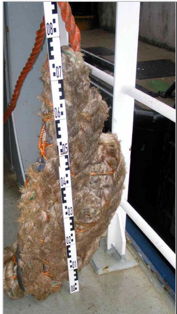
Figure 7: Fender – similar to the fender that was carried away
