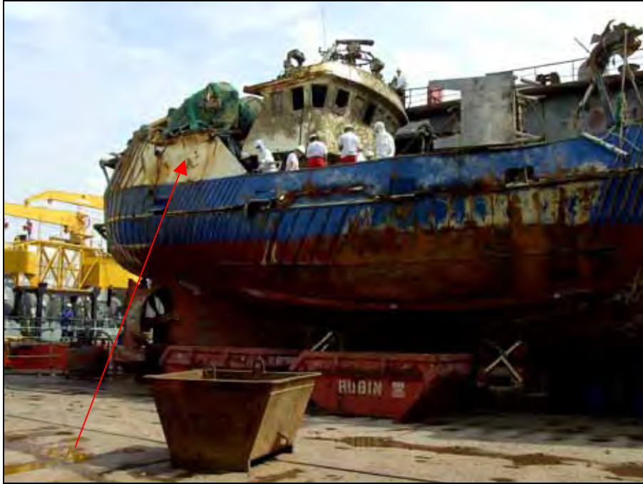
Figure 43: Net winch on the poop deck
