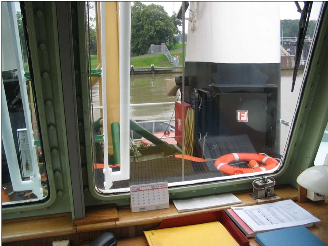
Figure 10: Field of vision of the tug master towards aft, if he makes one step from the control position to starboard
