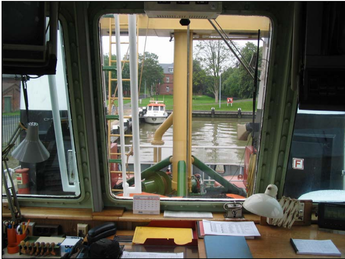
Figure 9: Field of vision of the tug master towards aft, limitation of the visibility by the funnels and the aft mast; above left the monitor
