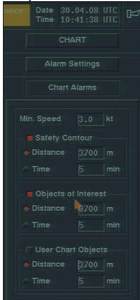
Figure 15: Menu for Chart Alarms on the Chartplot (later simulation)
