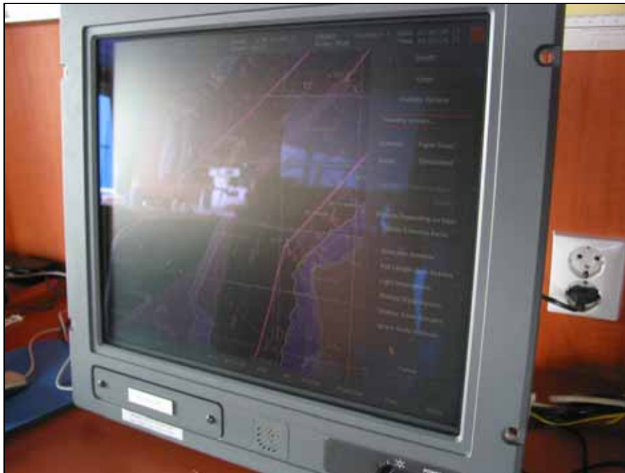
Figure 11: Second Chartpilot as a planning station at the chart table
