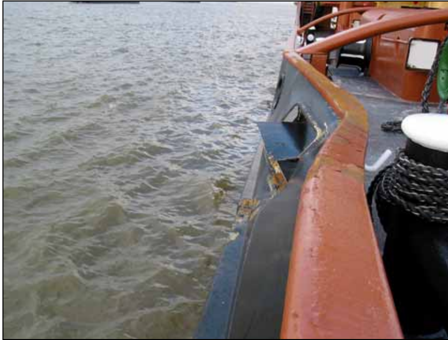
Figure 9: Damage to upper deck on the port side of OCEANIC
