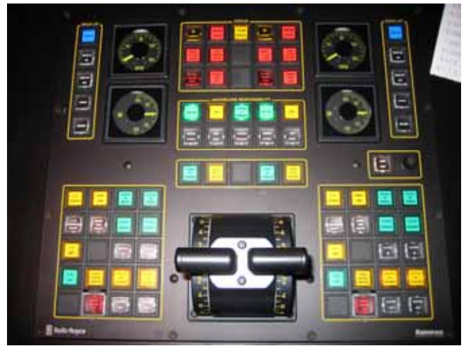
Fig. 2: Bridge wing conning station - main propulsion monitoring panel including drive lever
