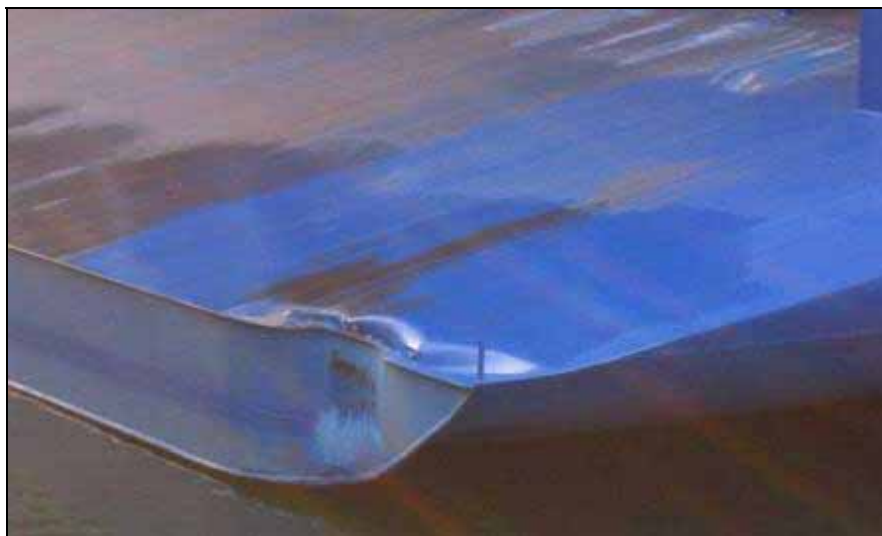
Figure 6: Damage to the transom on the starboard side of the FINNLADY
