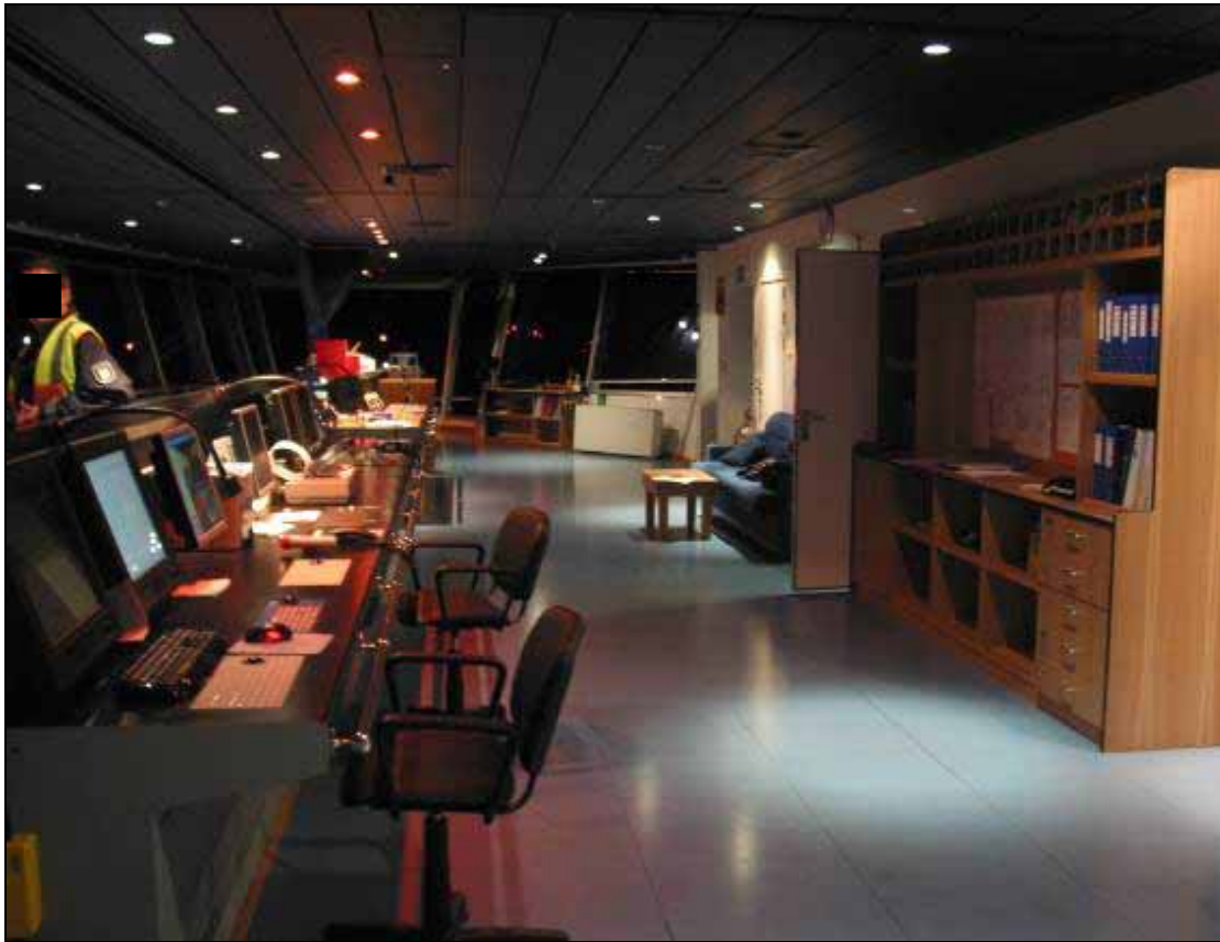
Figure 13: Wheelhouse with integrated starboard wing
