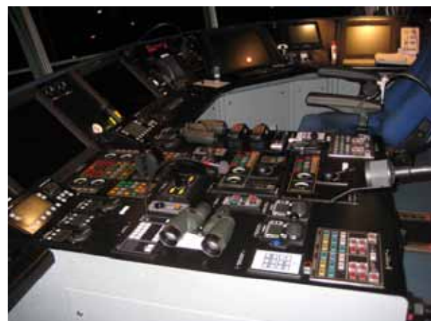
Fig. 8: Central bridge conning station - details
