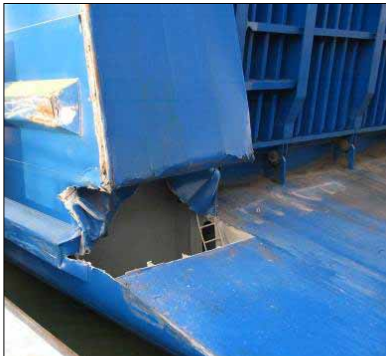
Figure 4: Damaged cofferdam on the port side of the FINNLADY
