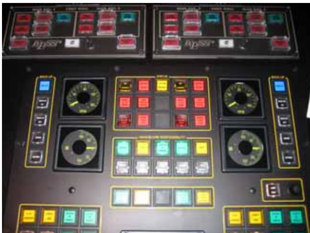
Fig. 3: Bridge wing conning station - main propulsion monitoring panel
