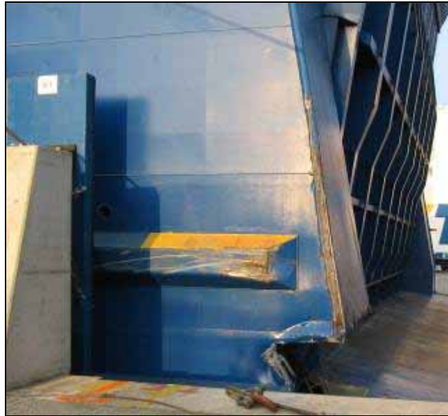
Figure 3: Damage to the port-side shell plating of the FINNLADY
