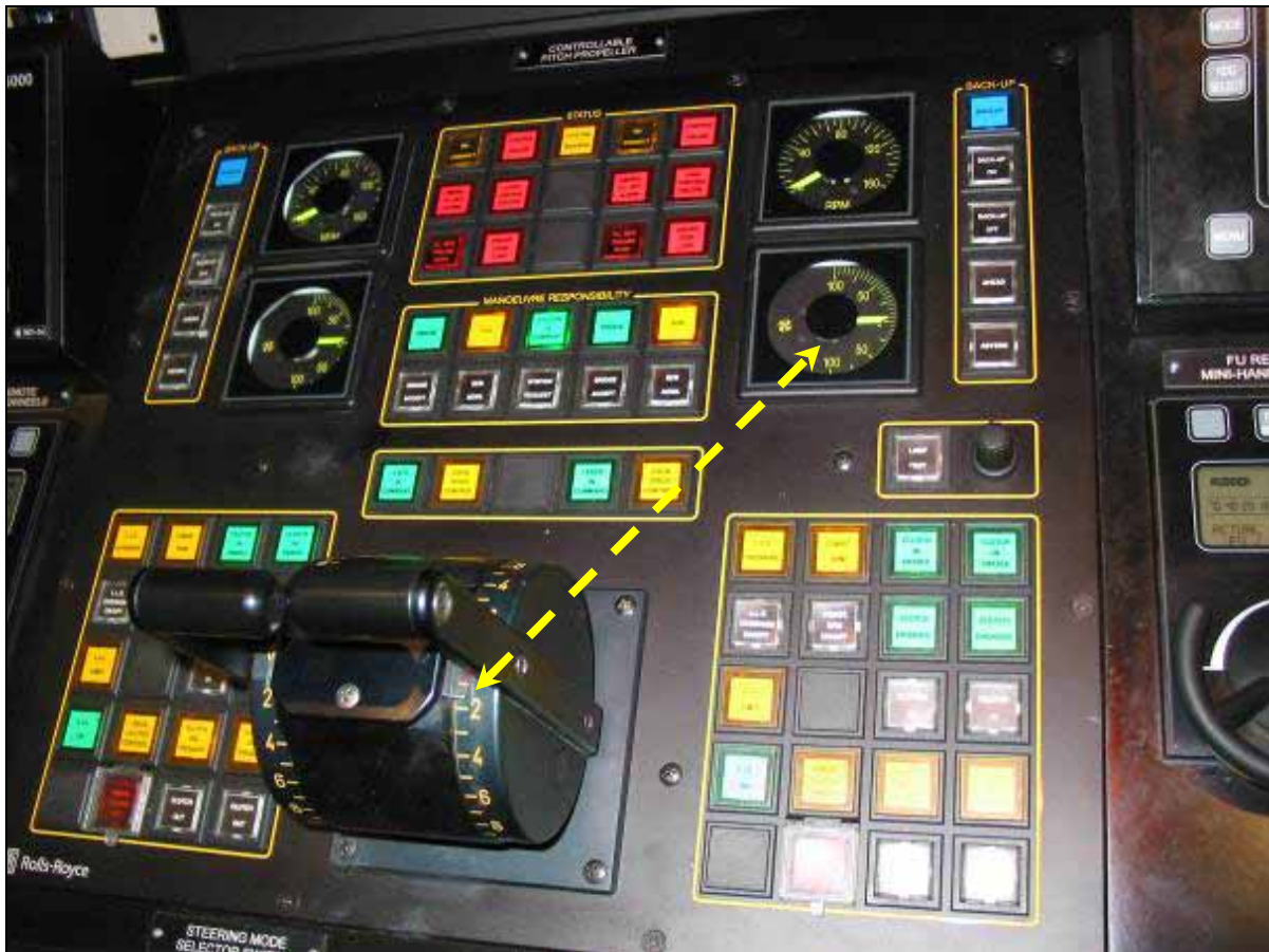
Figure 31: Analogue pitch display and control lever on the bridge
