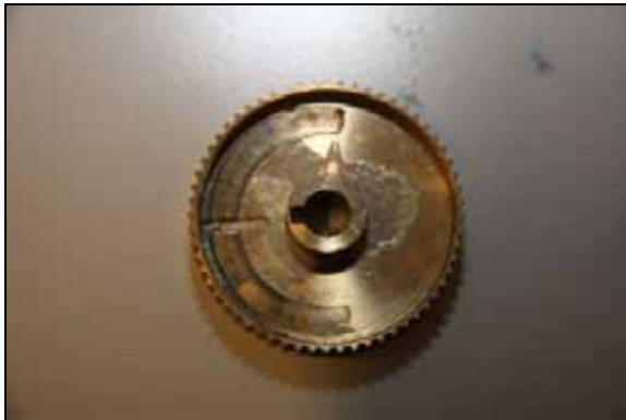
Figure 15: Cog Wheel with groove
