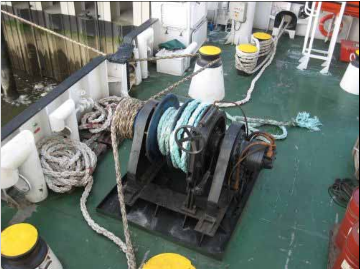
Figure 8: Port Winch with Broken Spring
