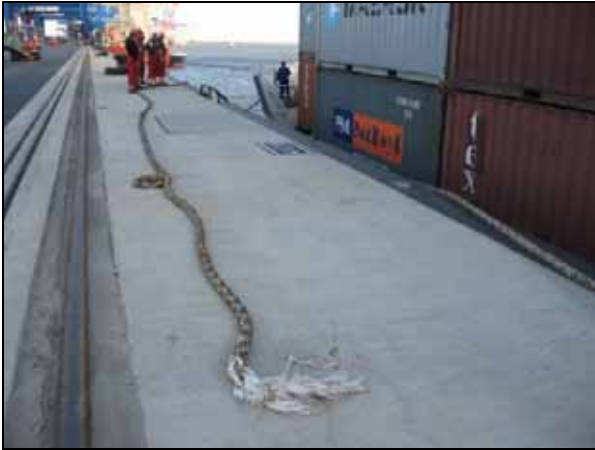
Figure 6: Broken Fore Spring Line
