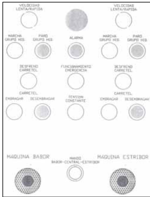
Figure 9: Operation Station for Winches amidships at the transom
