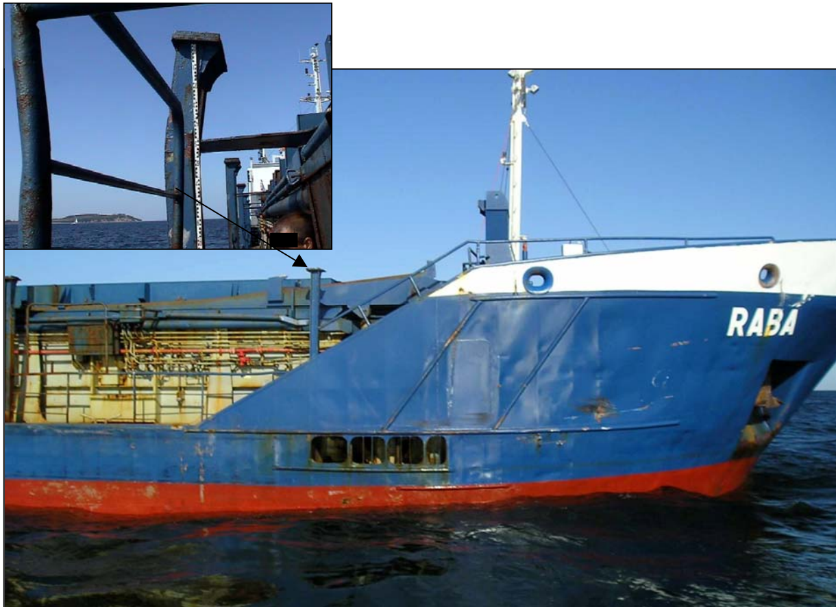
Figure 5: Damage to the bow of the RABA
