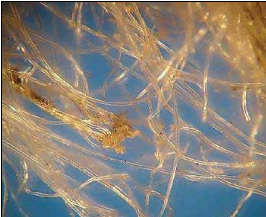
Photograph 7 Fused filaments from core fail point of figure 1
