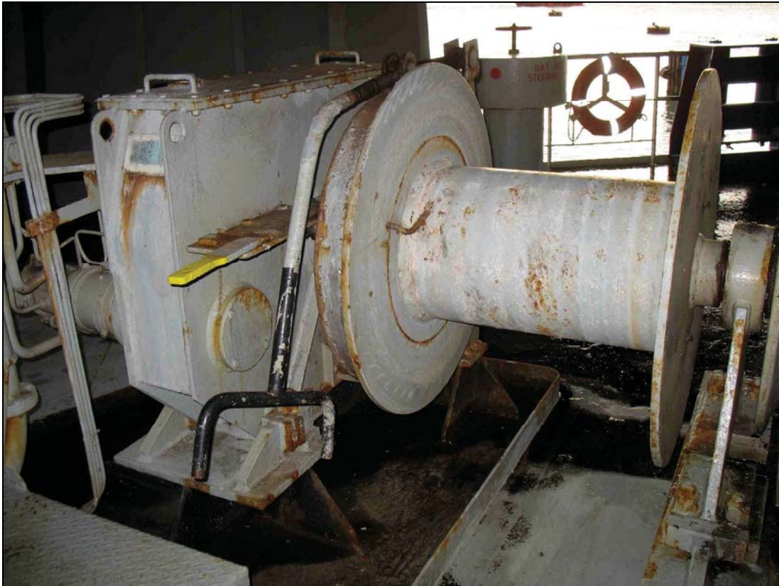
Figure 4: Bent brake rod on the port winch
