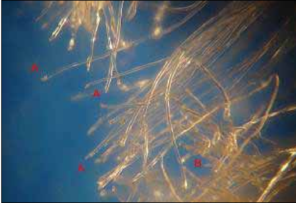
Photo 9 Failed filaments from inner rope yarns of core assembly
