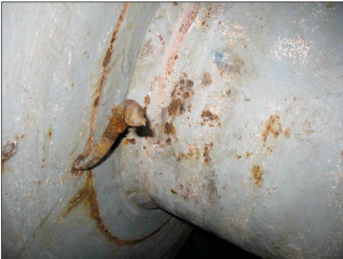
Figure 5: Ripped out bolt pin for holding the line end on the winch drum
