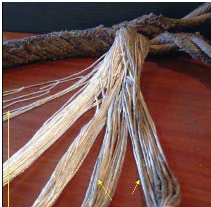
Photograph 14 'Clear of fail zone' sample unraveled to expose core rope yarns
