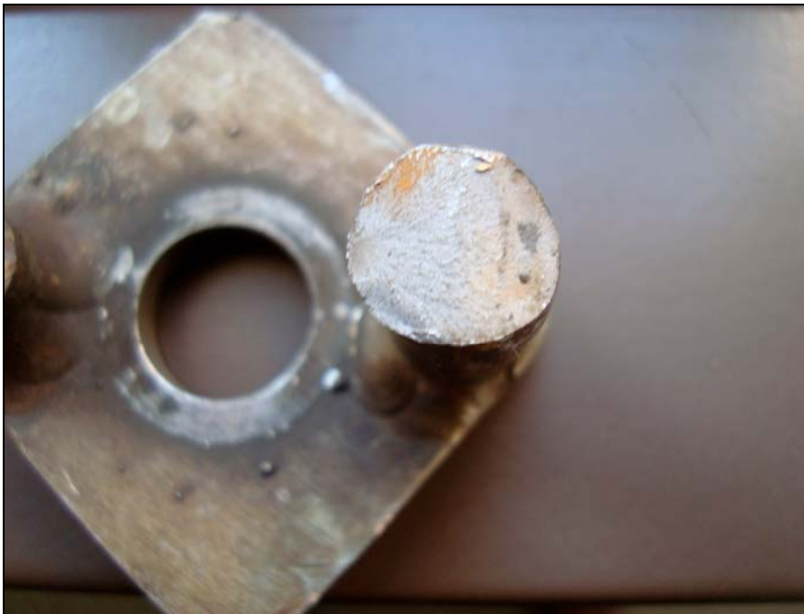
Figure 15: Close-up of the secondary fracture surface
