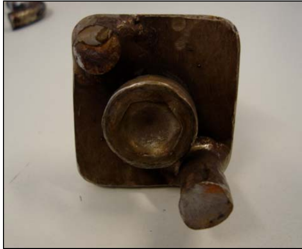
Figure 12: Ring mounting (top view of fracture)
