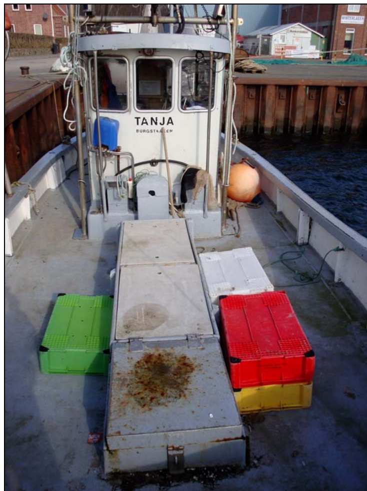
Figure 3: Cover of fish compartment with extended bearing surface
