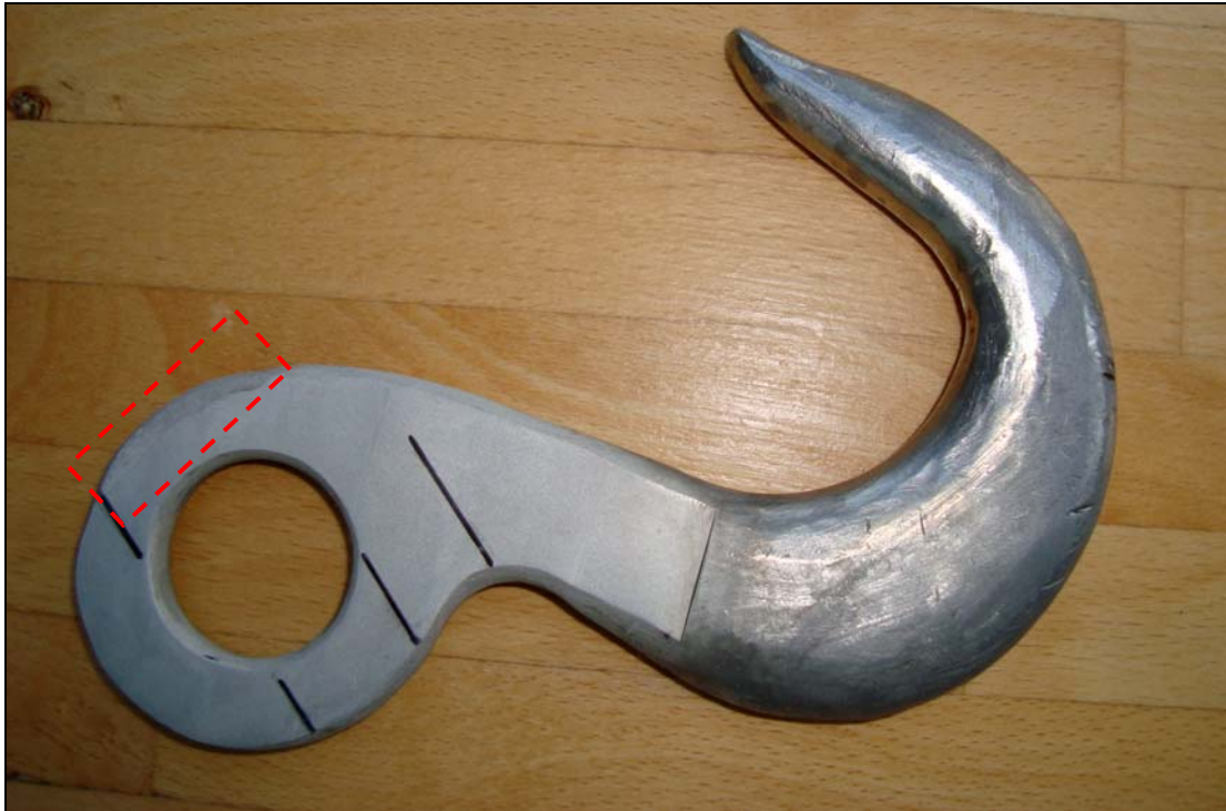
Figure 21: Hook with corrective weld (outlined in red) and rolling direction 8
