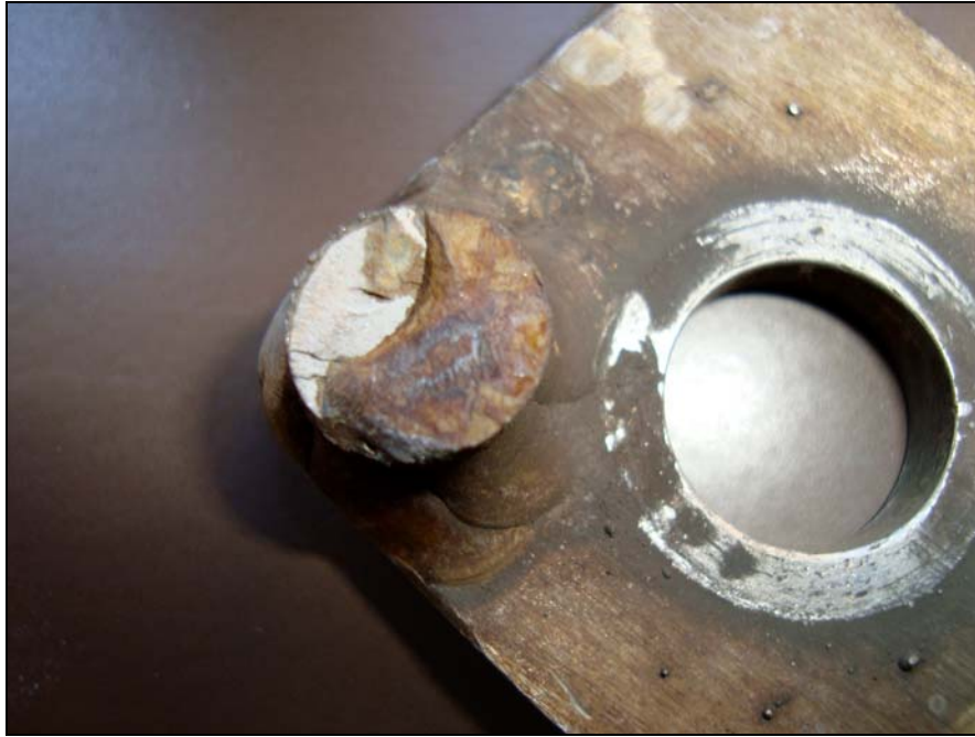
Figure 14: Close-up of the primary fracture surface
