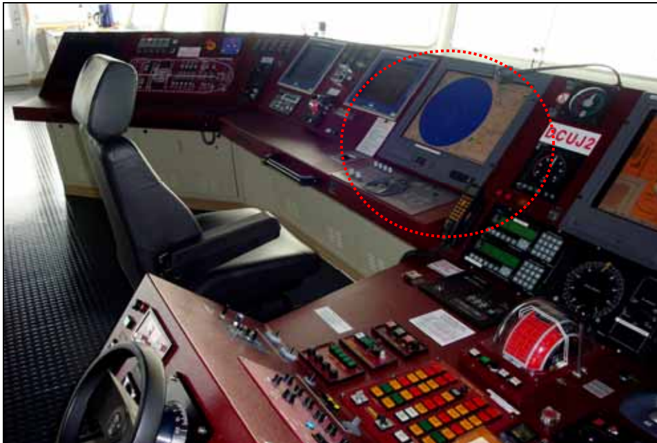
Figure 38: Extract – bridge console with port radar unit
