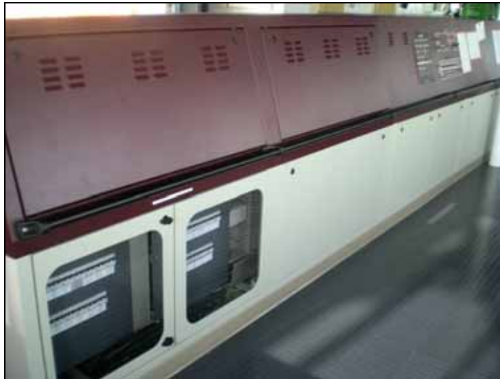
Figure 43: Handrail on the forward edge of the chart table
