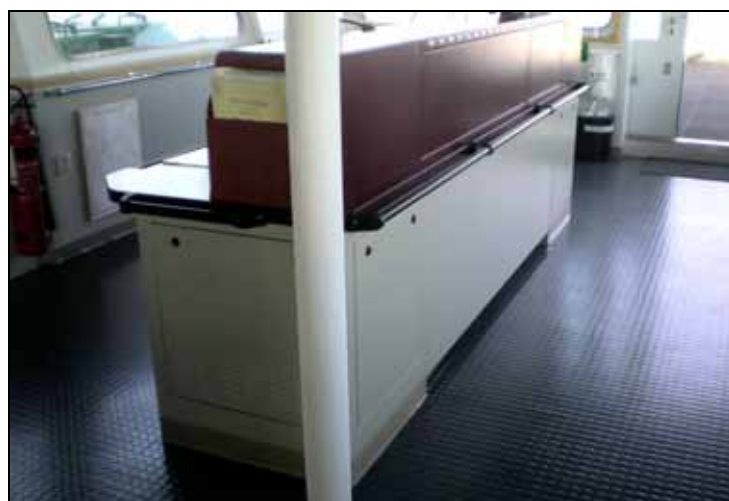
Figure 44: Handrail on the forward edge of the GMDSS console
