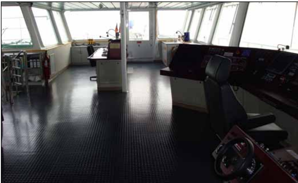
Figure 21: No handrails at the port side of the bridge
