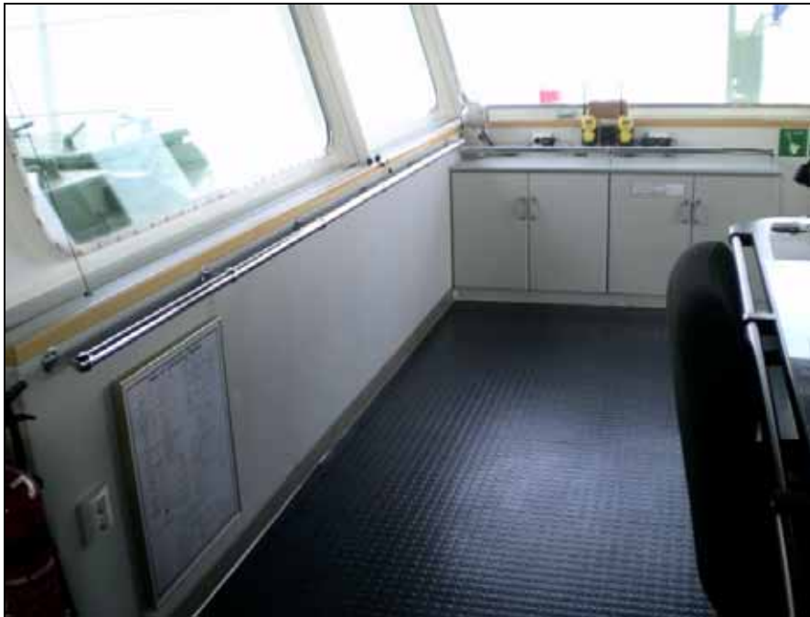
Figure 45: Handrail on the port side and aft end of the bridge
