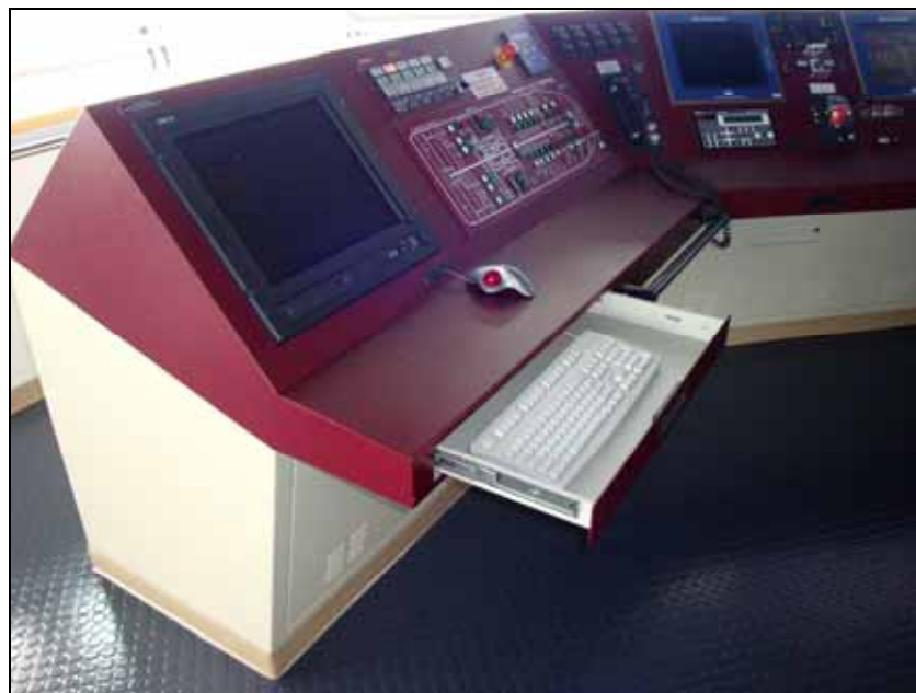
Figure 17: Bridge console inadequately equipped with handrails
