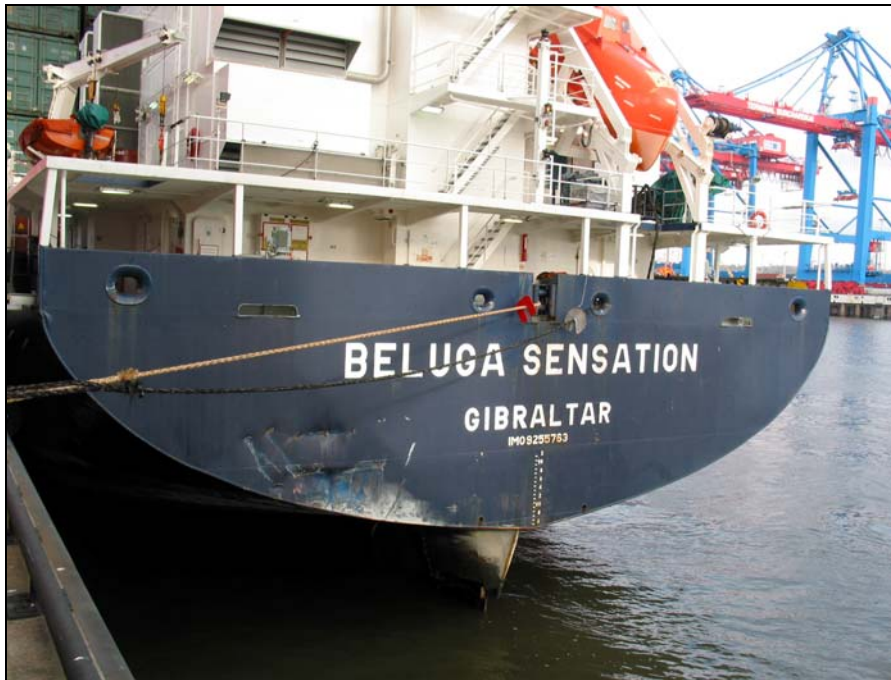
Figure 3: BELUGA SENSATION, damage to stern
