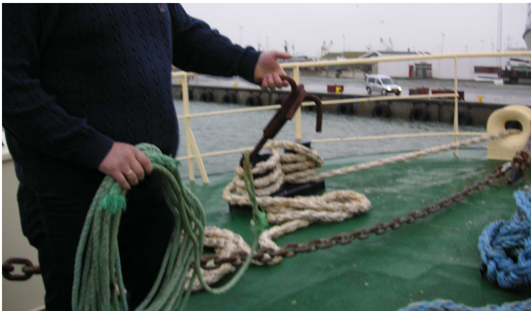
A fisherman holding the grapnel and the grapnel line. Photo by the Investigation Division
