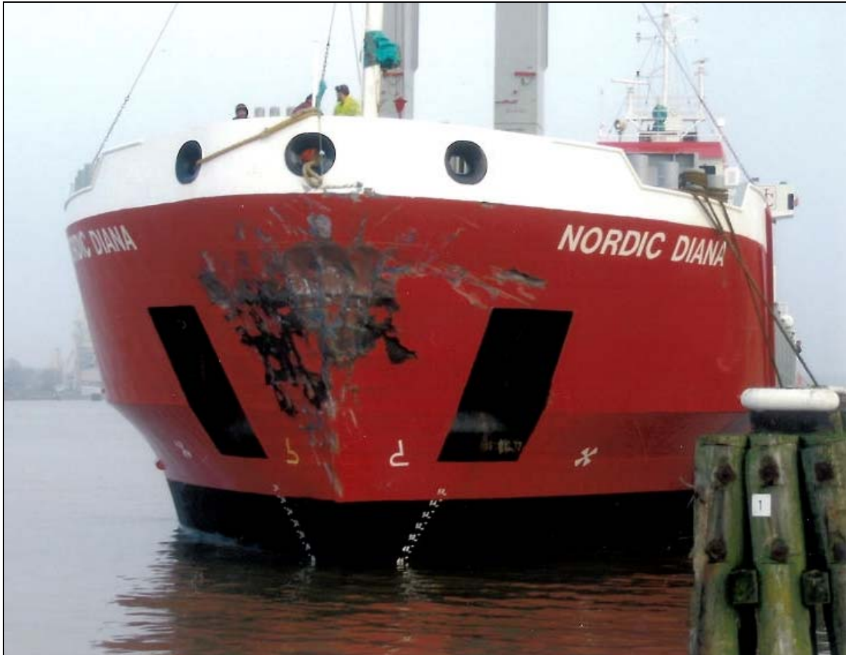
Figure 5: Damage to the MV NORDIC DIANA
