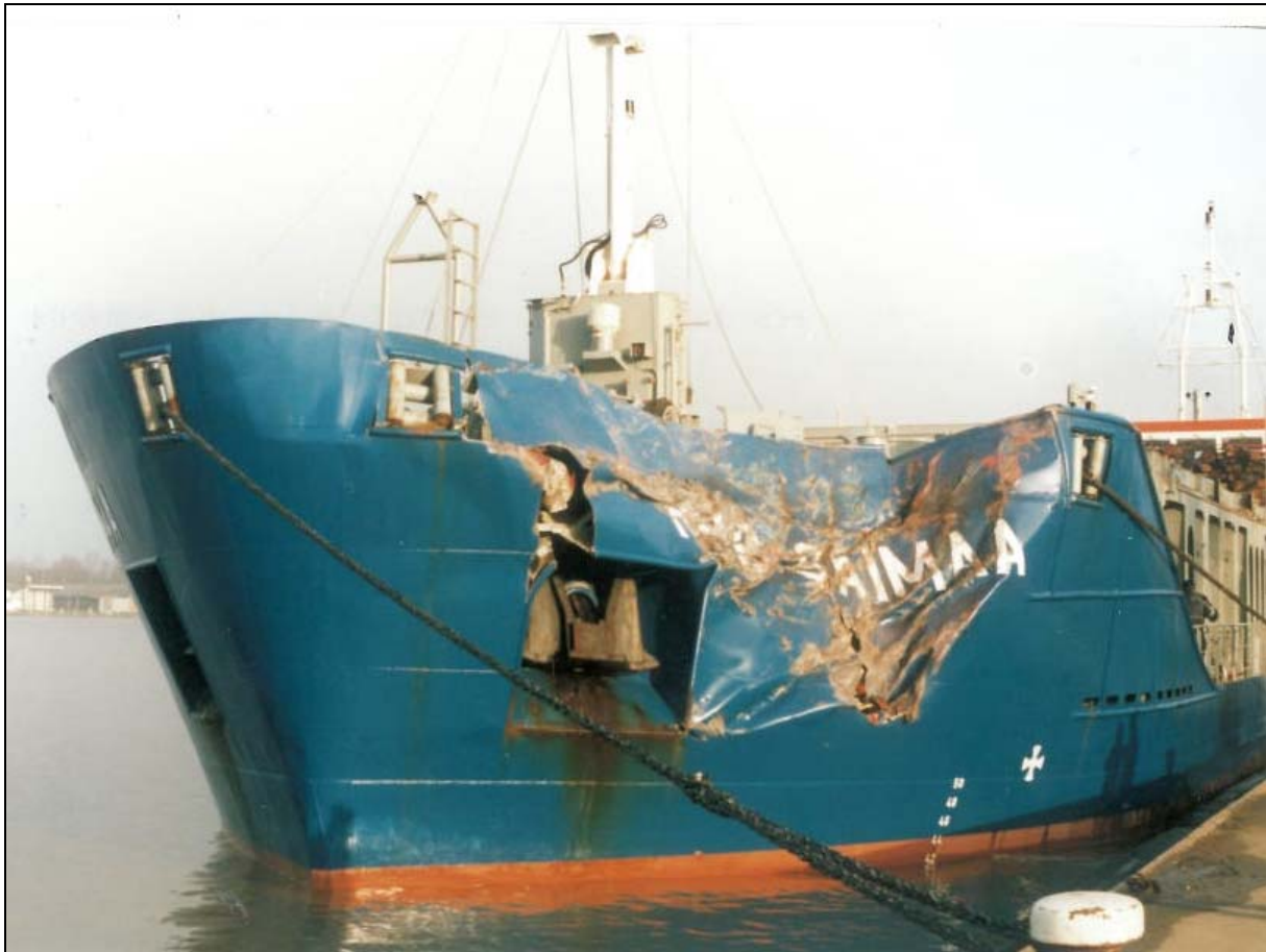
Figure 6: Damage to the RMS SAIMAA
