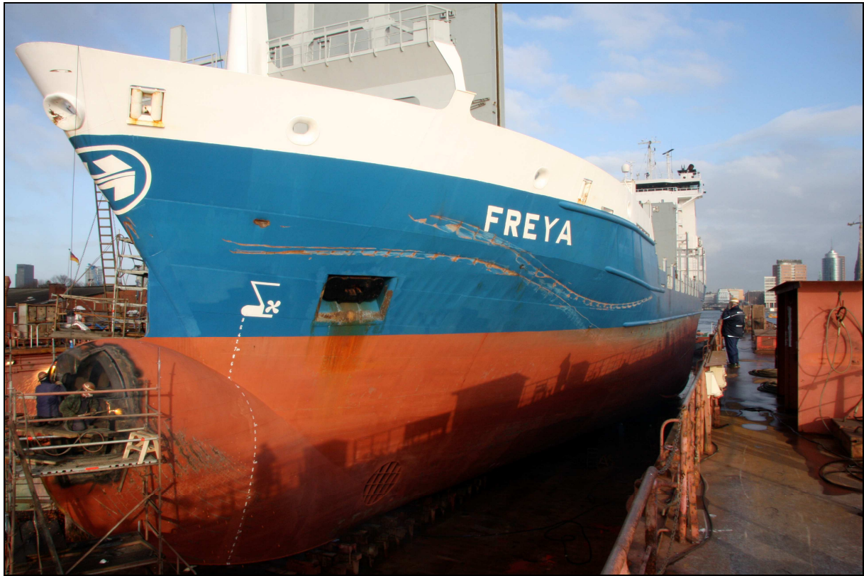
Figure 5: Damaged port side of the FREYA
