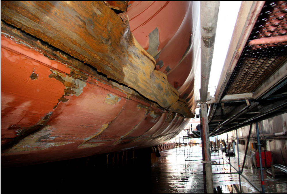
Figure 7: Damaged underwater hull of the FREYA
