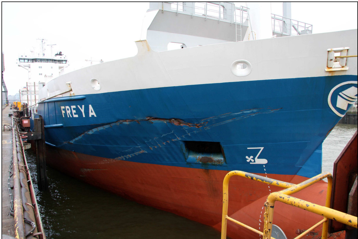
Figure 3: Damaged starboard side of the FREYA
