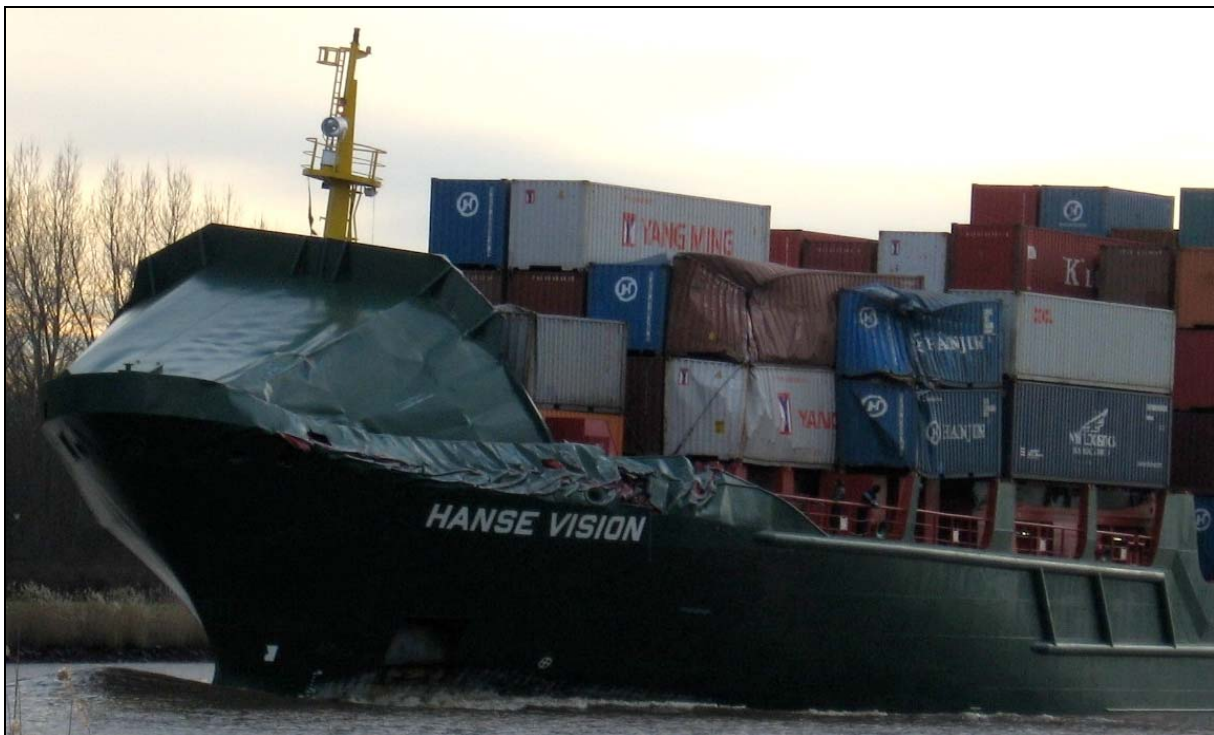
Figure 8: Damage detail HANSE VISION
