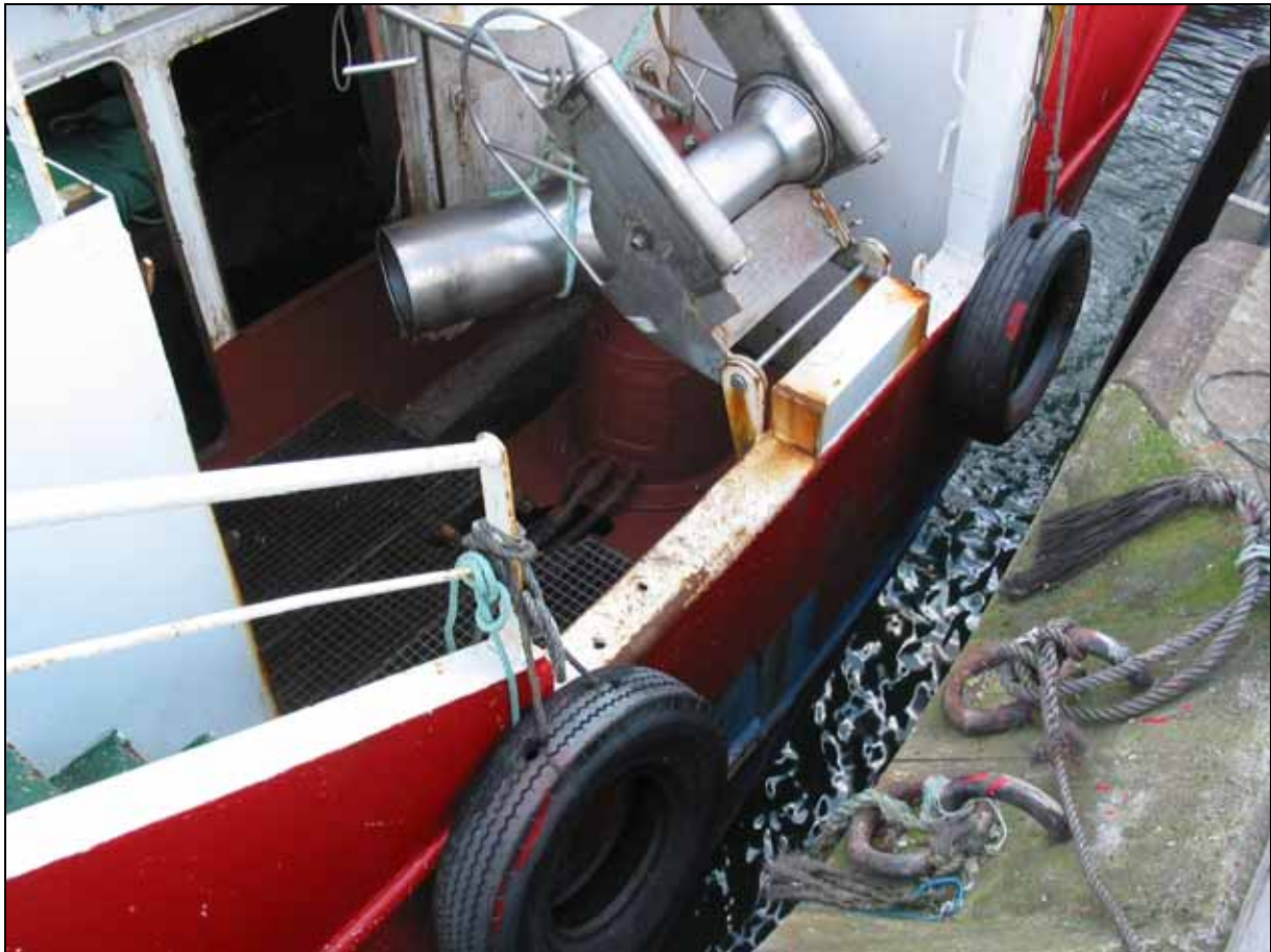
Figure 11: Access to the upper fish processing area on the starboard side. The opening is behind the bulwark. The net is deployed through the smaller opening; the larger one is used to enter the fish hold.
