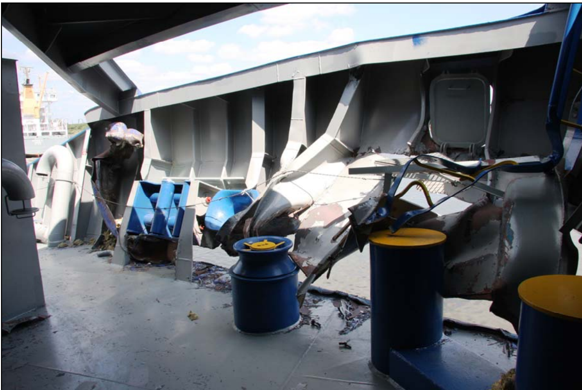
Figure 7: TRANSANUND, damage to the forecastle
