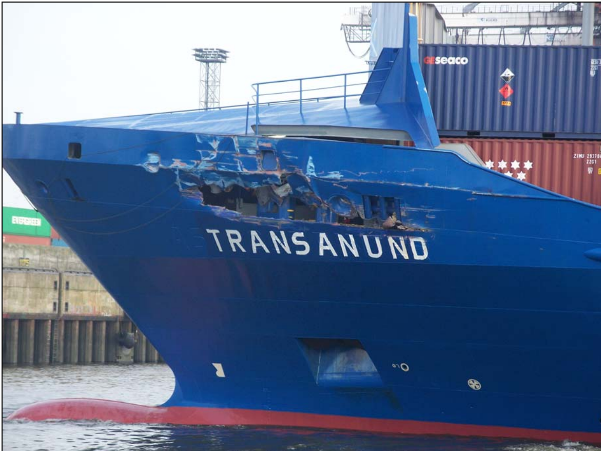
Figure 6: TRANSANUND, damage to the forecastle
