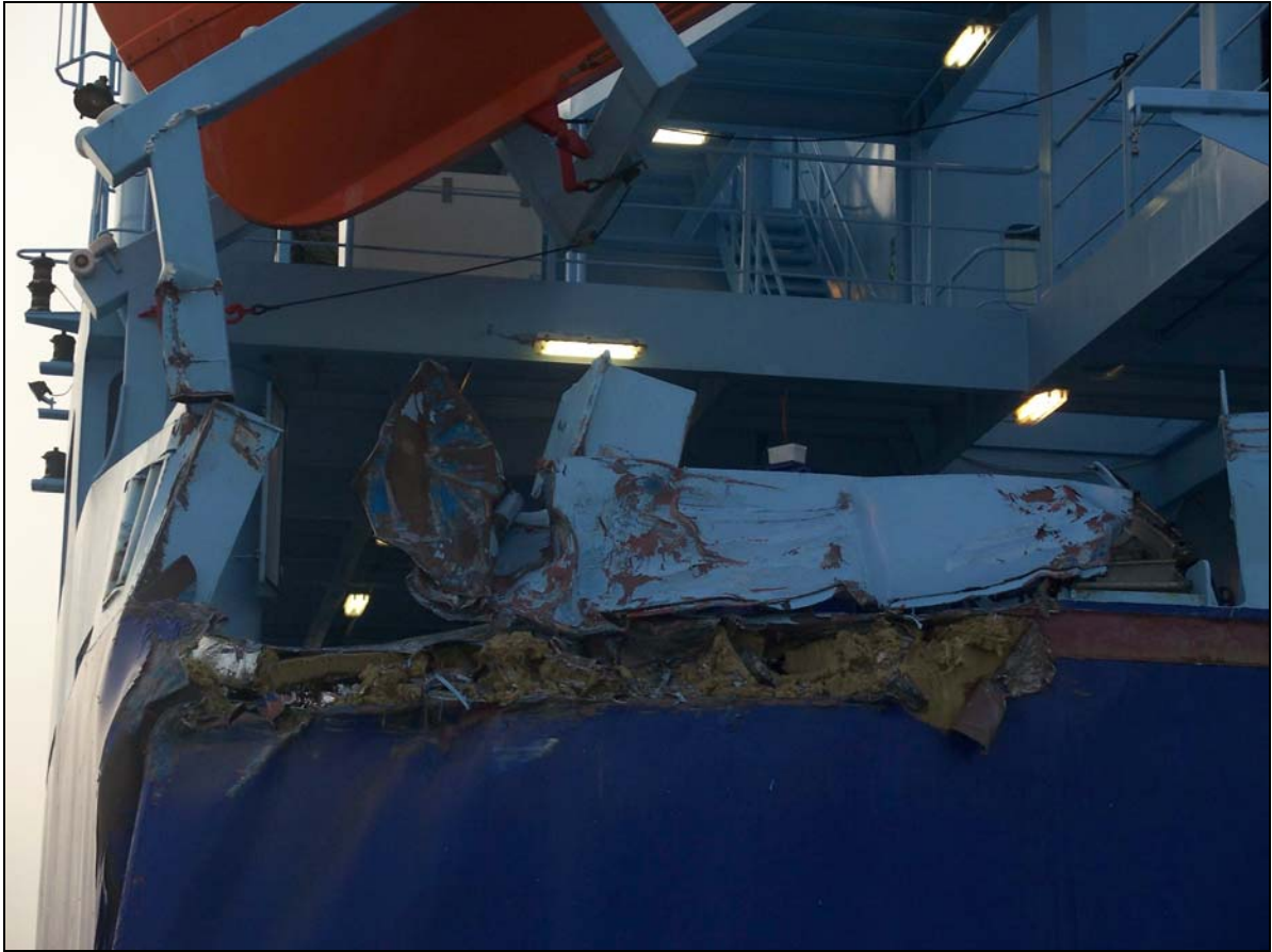
Figure 4: AURORA, damage at the stern
