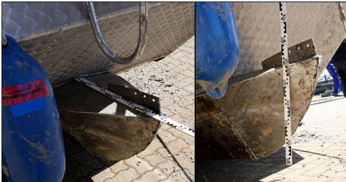
Figure 8: Keel design of the QUINTETT, view from fore
