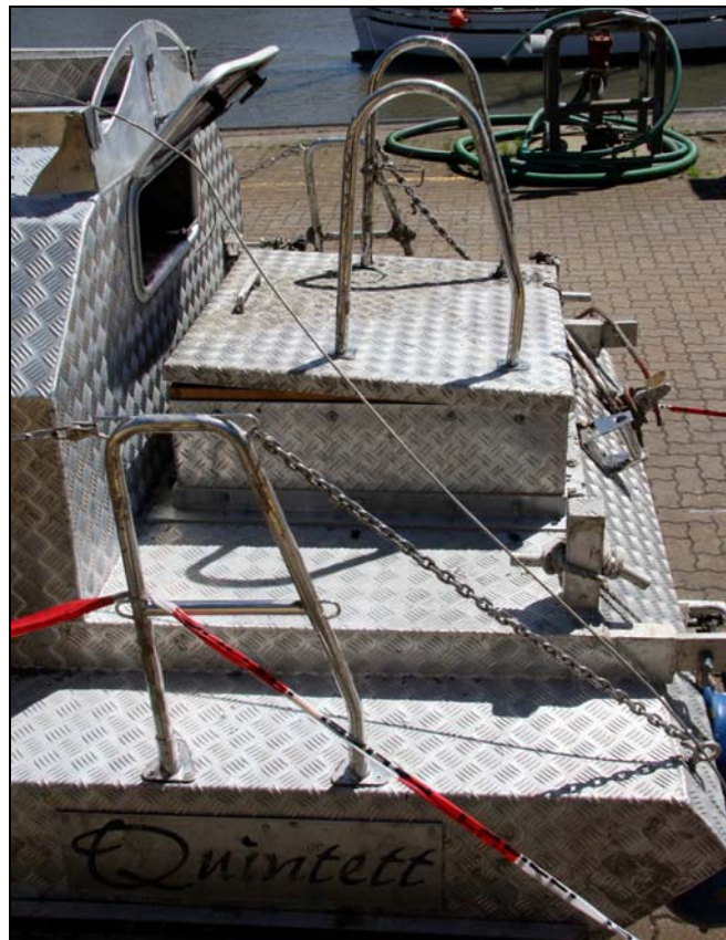
Figure 21: Hatch on the foredeck of the QUINTETT, closed
