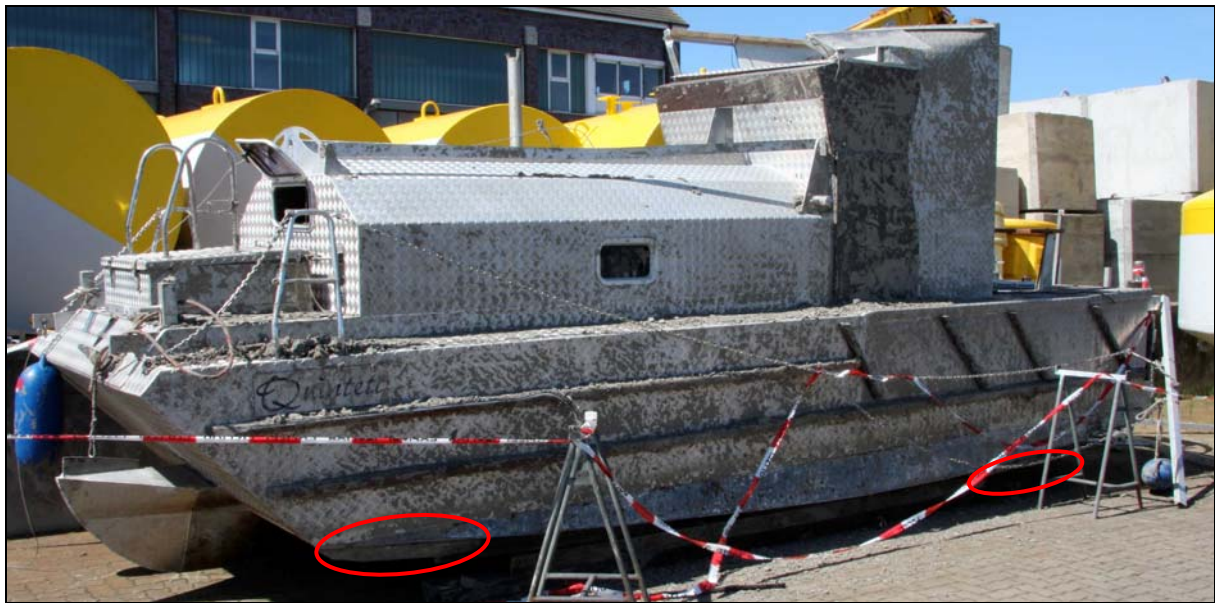
Figure 11: Arrangement of the bilge keels on the port side
