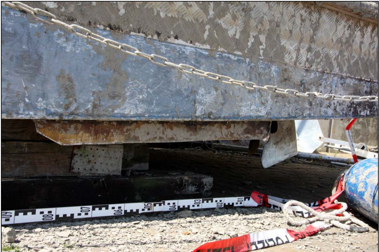
Figure 10: Bilge keel, aft port side, side view
