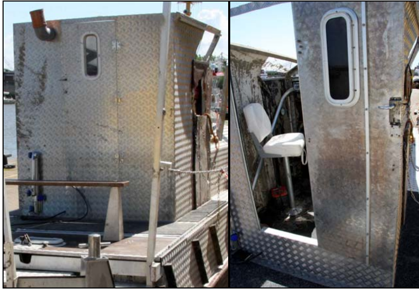
Figure 17: Access door to the wheelhouse
