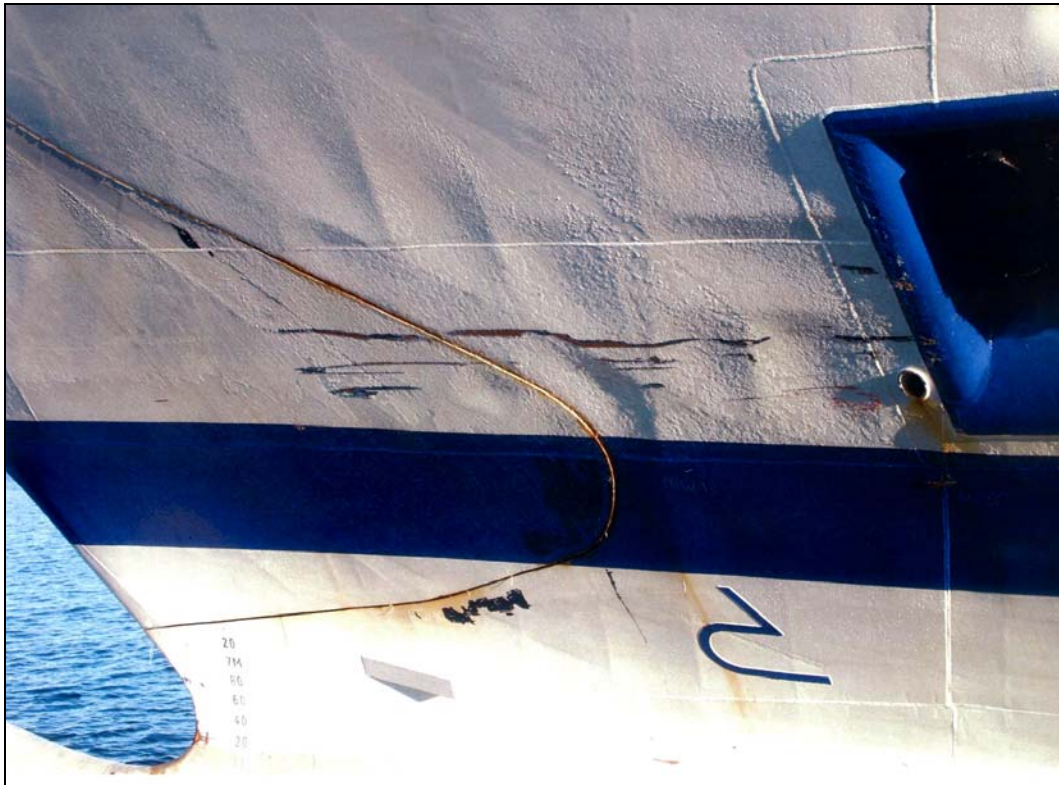
Figure 5: Paint abrasions on the stem of the MF SKANIA 9
