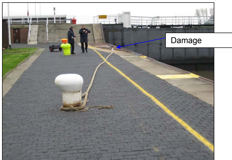
Figure 4: Broken mooring line laid out
