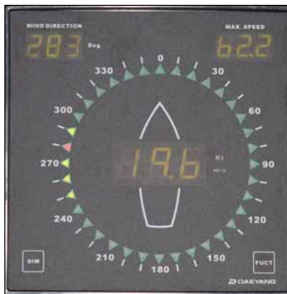
Figure 39: Display of the wind force and direction on the bridge of the HÖEGH LONDON at the time of the survey by the BSU; display of the wind force in knots (slightly backlit)
