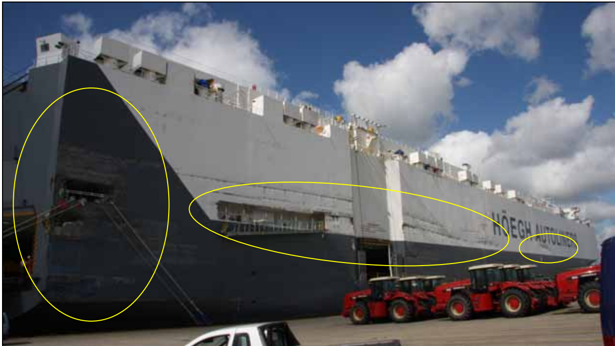
Figure 5: Side view of the HÖEGH LONDON with dents
