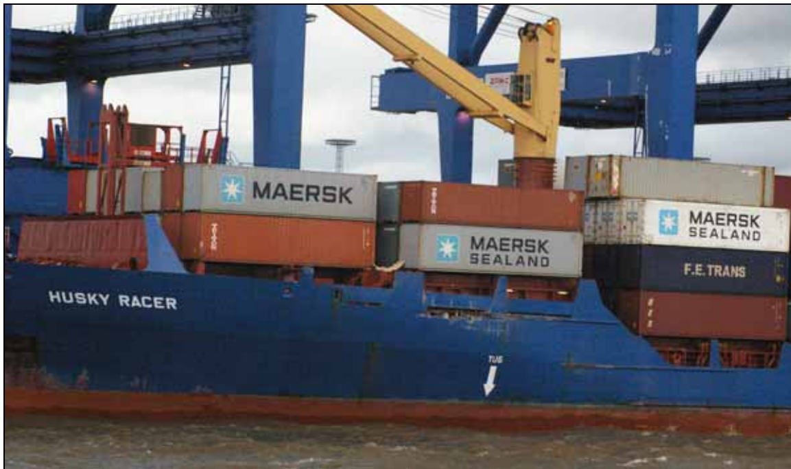
Figure 9: HUSKY RACER, damaged hull, twisted crane
