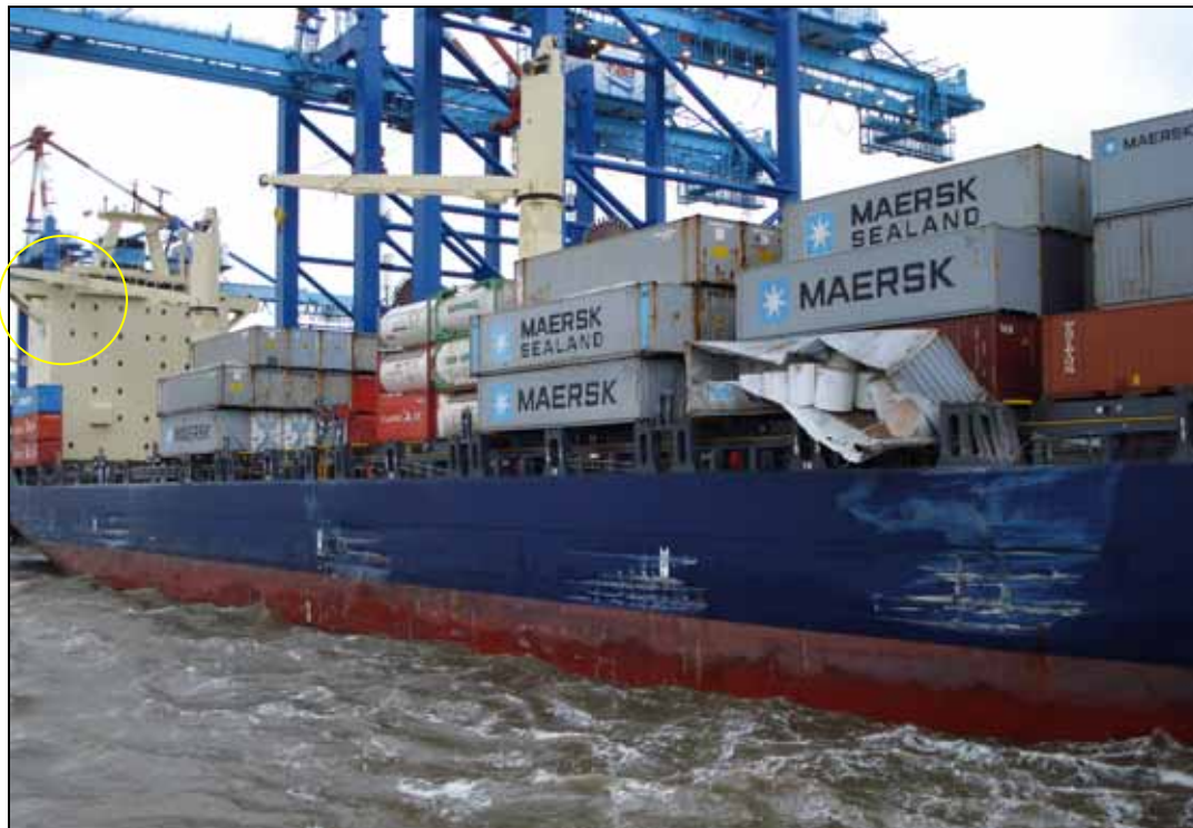
Figure 6: MAERSK NEWARK, damaged hull, twisted and damaged cranes
