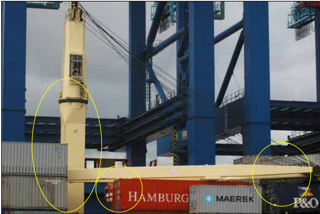
Figure 7: MAERSK NEWARK, crane jib of crane number 1 torn off and damaged container
