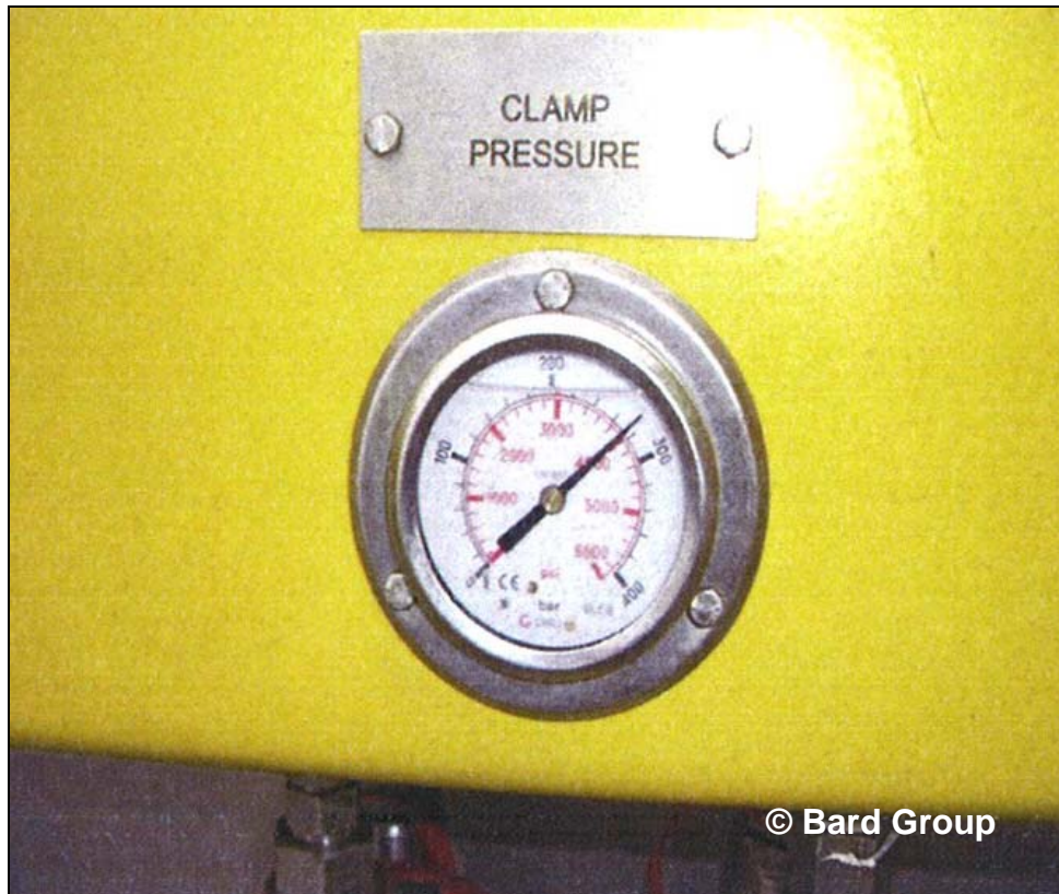
Figure 22: Analogue pressure gauge on power pack 36
