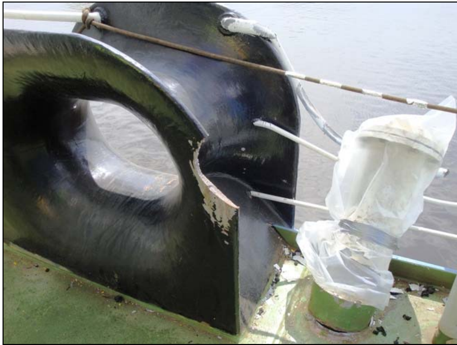
Figure 6: Damage to a fairlead caused by flying debris
