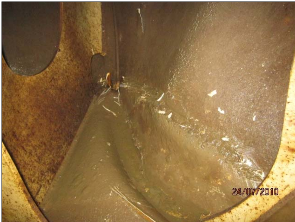
Figure 8: Damage to the forepeak of the JULA S 16
