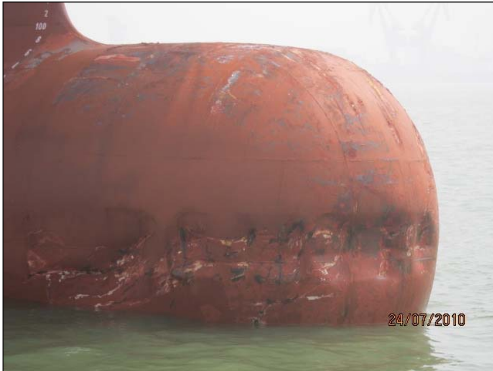
Figure 7: Damage to the bulbous bow of the JULA S 15
