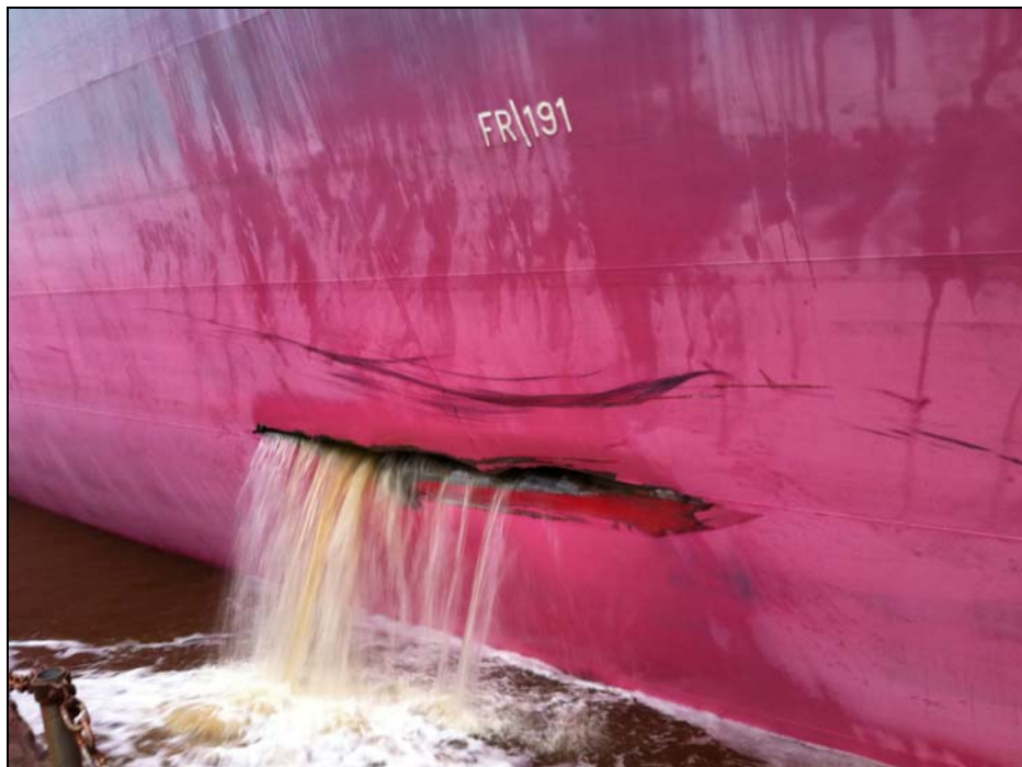
Figure 7: Damage photo 3 – FRISIA ROTTERDAM
