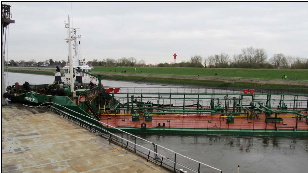
Figure 14: Front end of floating dock wedged into forecastle of the ZAPADNY (2)
