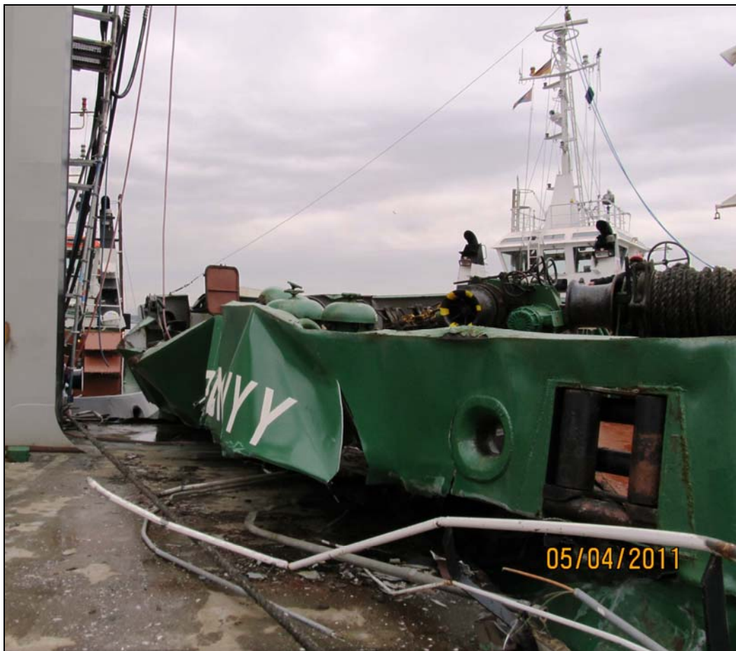
Figure 15: Damage to the forecastle of the TMV ZAPADNY (1)
