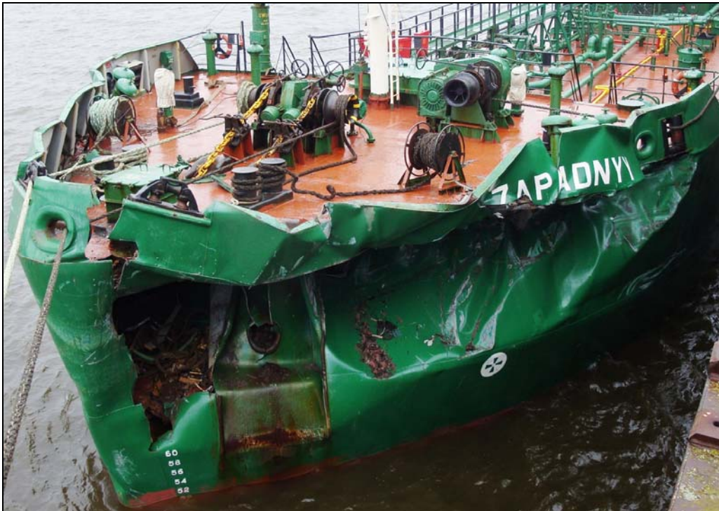
Figure 16: Damage to the forecastle of the TMV ZAPADNYI (2)
