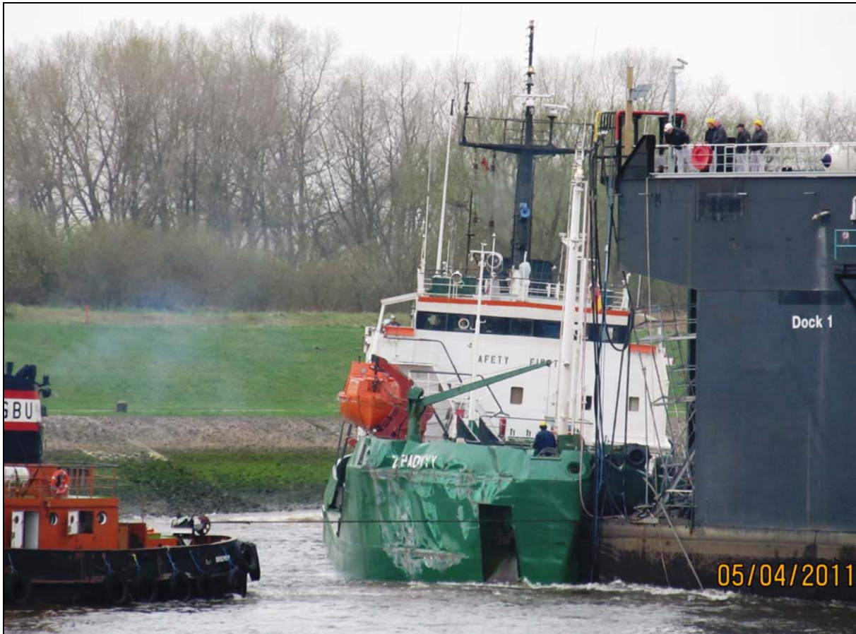
Figure 13: Front end of floating dock wedged into forecastle of the ZAPADNY (1)
