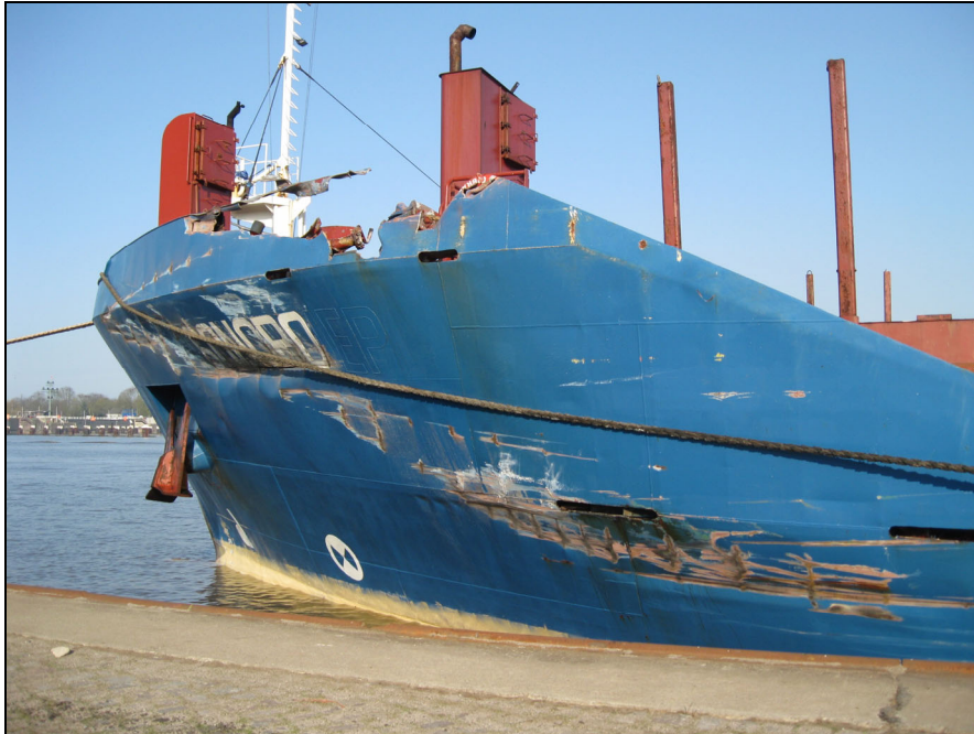
Figure 4: Damage to the bow of the SONORO
