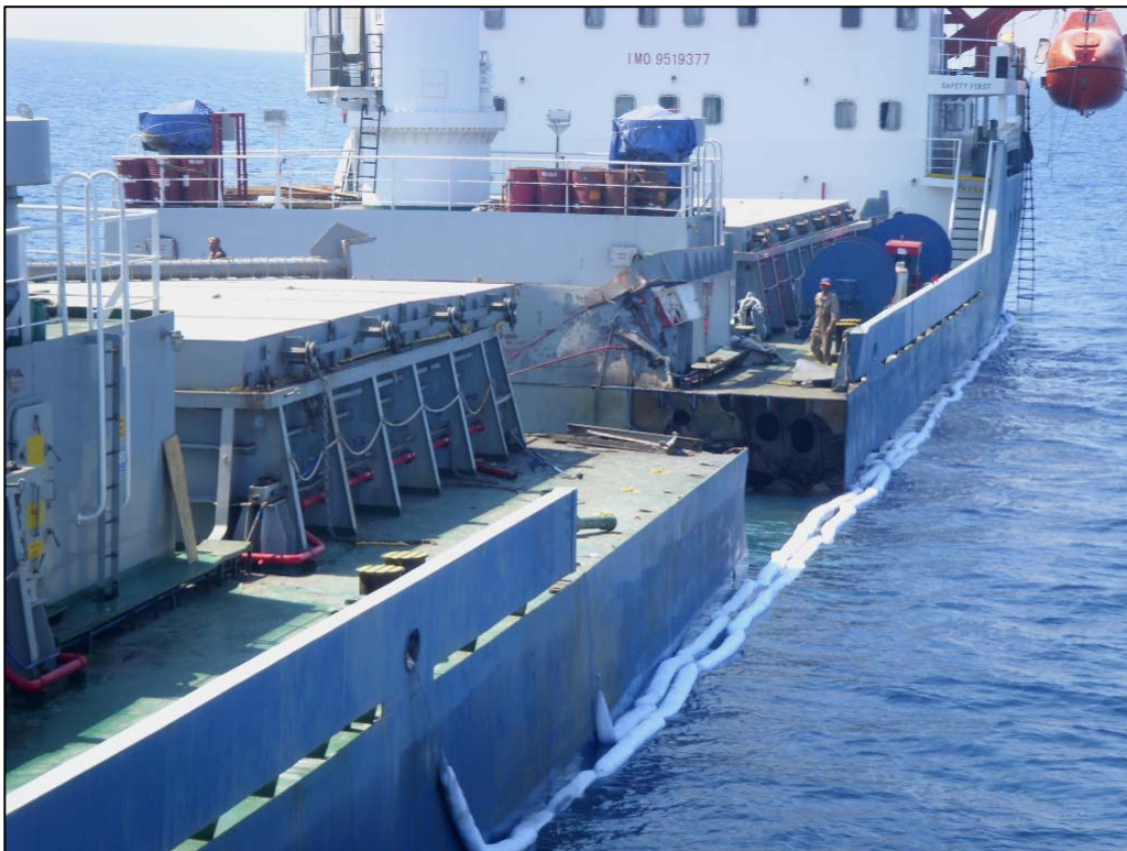
Figure 1.6iv: Marti Princess sustained most of her damage i.w.o. cargo hold no. 2 and down to 1500 mm above the BL
