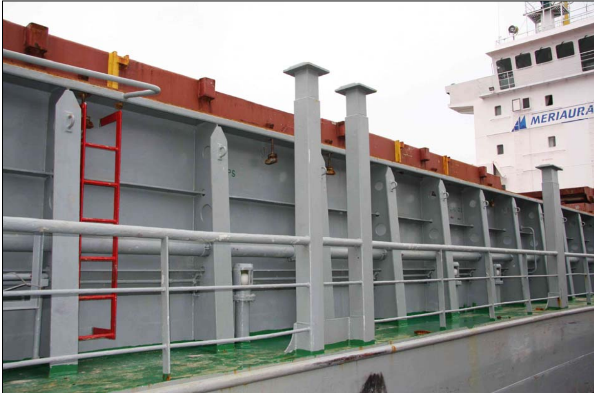
Figure 9: Ladder with rail
