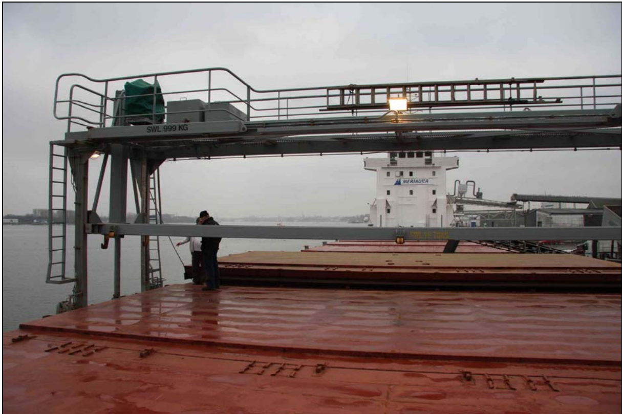
Figure 4: Gantry crane, platform and control position
