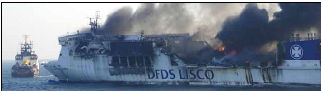
Figure 116: Fire on the weather deck and partially collapsed superstructure, taken on 9 October 2010 at 1645
