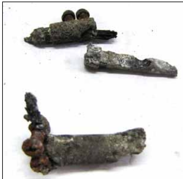
Figure 96: Remains of the contact pins found between truck and trailer
