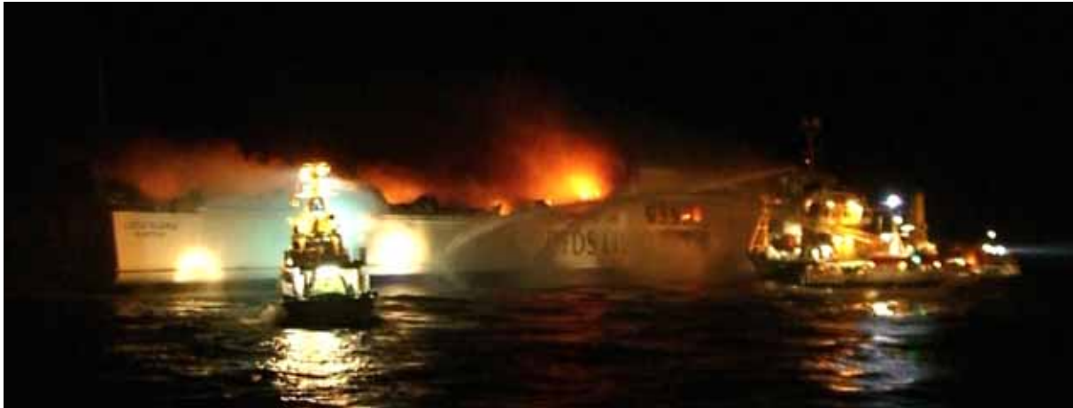
Figure 6: Cooling the shell plating of the LISCO GLORIA on the morning of 9 October 2010
