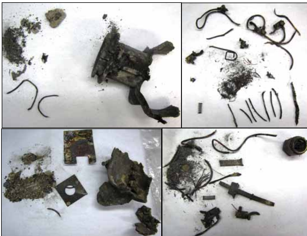
Figure 94: Remains of two switchable multiple sockets
