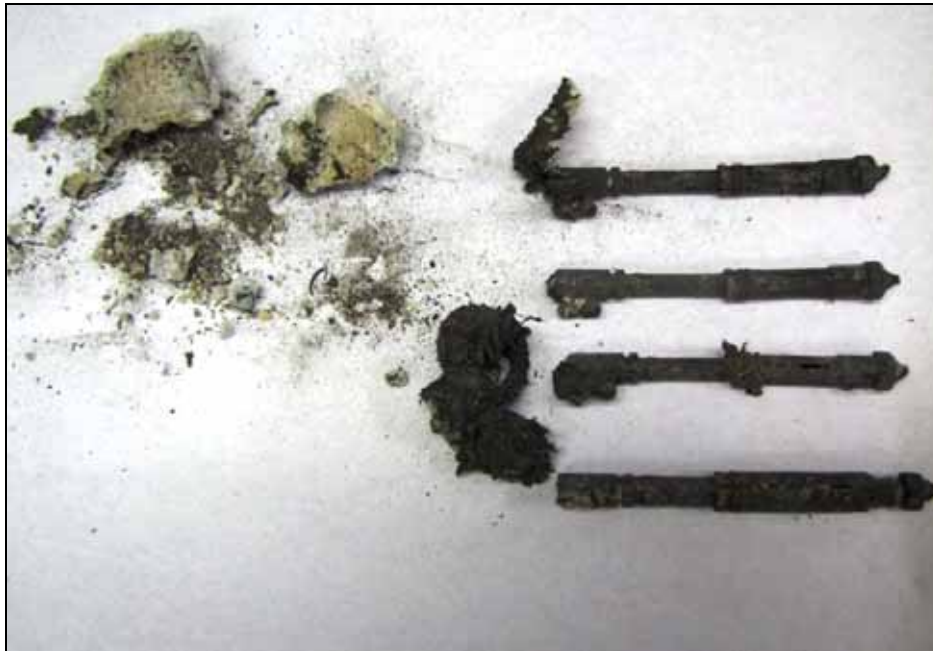
Figure 95: Remains of the contact materials of the plug-in connectors
