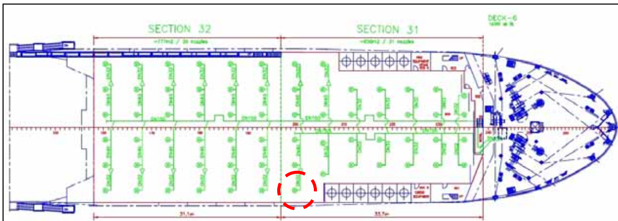
Figure 79: Drencher sections on the upper deck of the LISCO GLORIA
