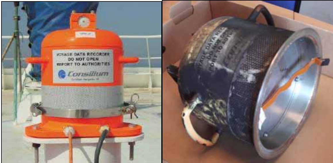
Figure 123: Capsule of the VDR in its original condition (model for comparison) and from aboard the LISCO GLORIA
