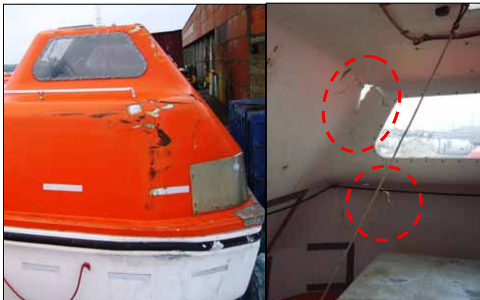
Figure 28: Damage to the stern of Lifeboat 1, view from outside and from inside
