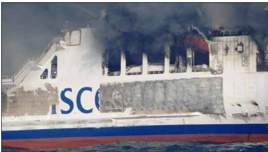
Figure 113: Material loss in the transition to deck 7, taken on 9 October 2010 at 1038
