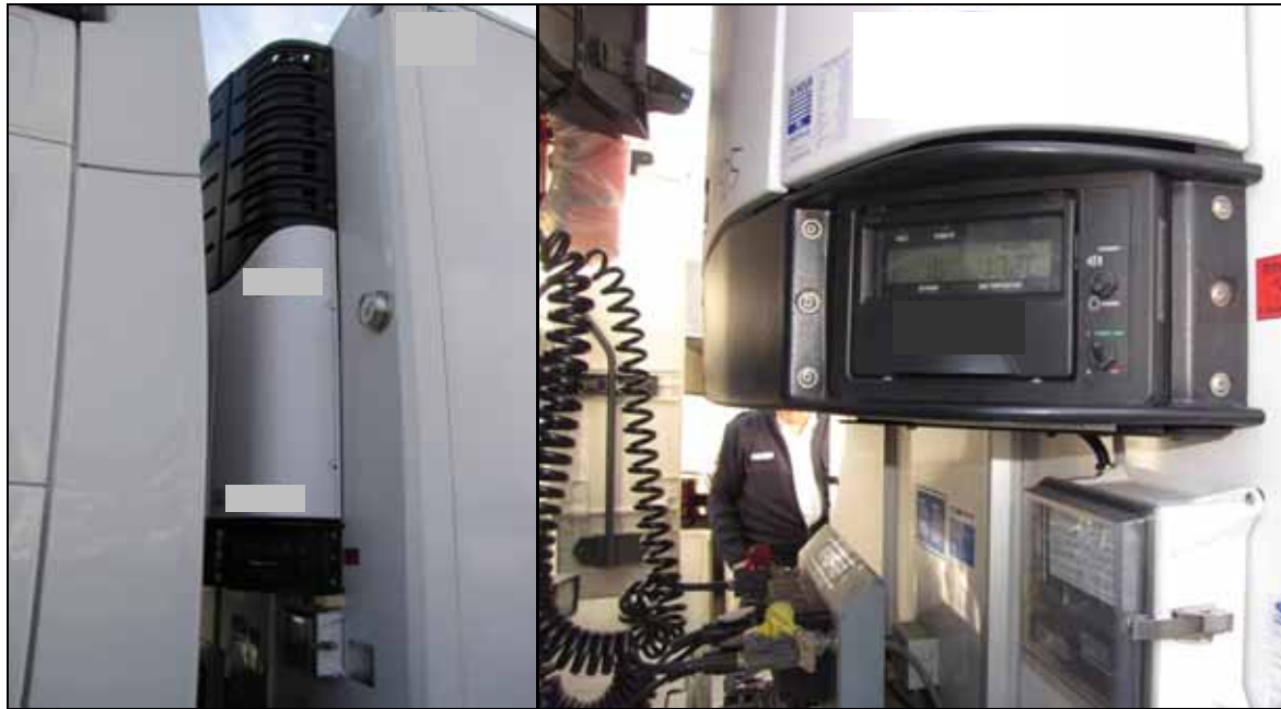
Figure 53: Refrigeration unit mounted between the cab and trailer
