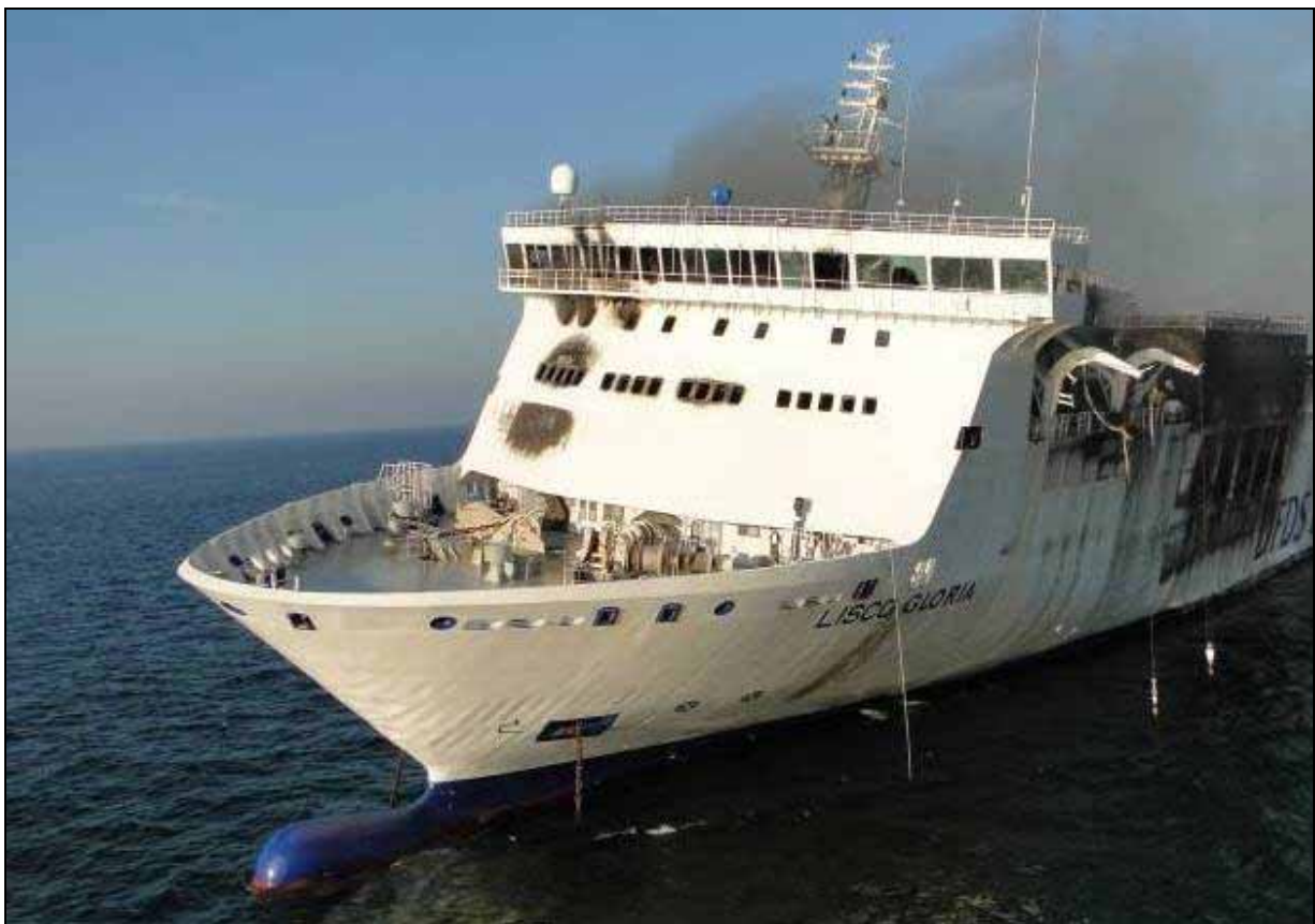
Figure 14: Hardly damaged forecastle of the LISCO GLORIA
