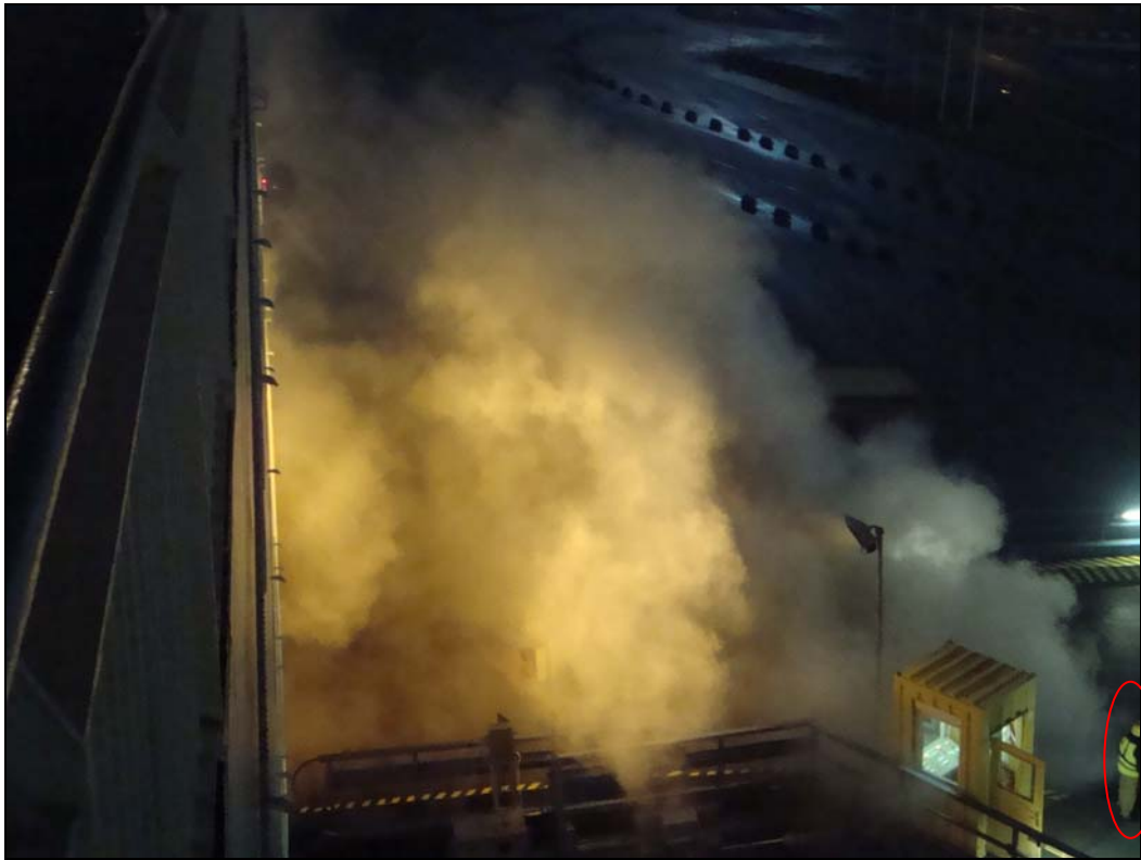
Figure 15: Build-up of smoke outside the vessel after the bow side door on deck 4 was opened 6
