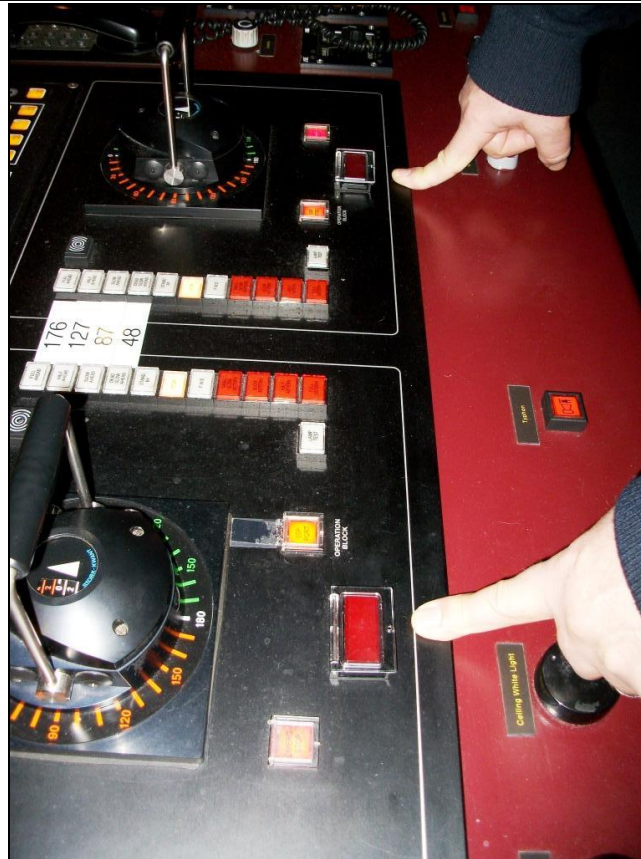
Figure 27: New position of the 'Crash stop' buttons below the control levers
