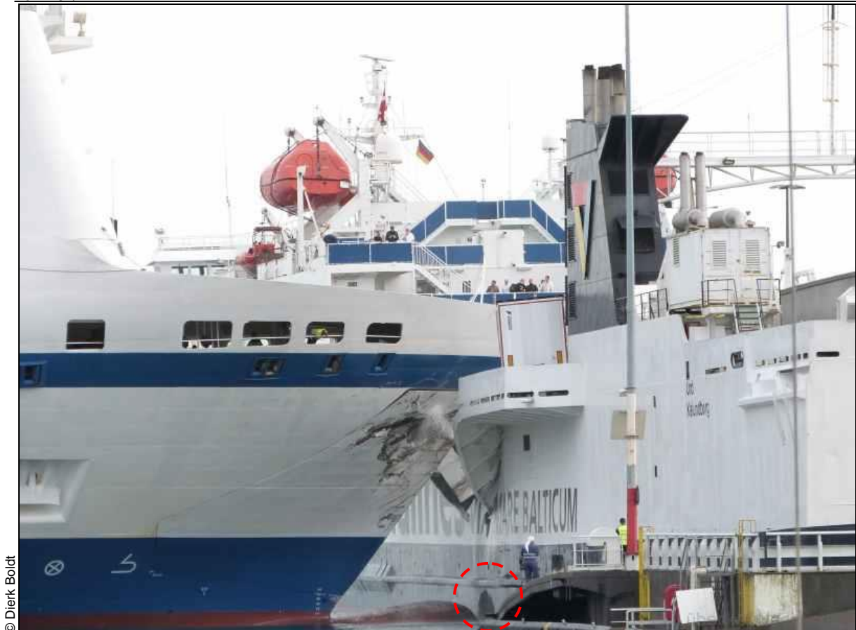
Figure 8: Photo taken shortly after the collision, close up
