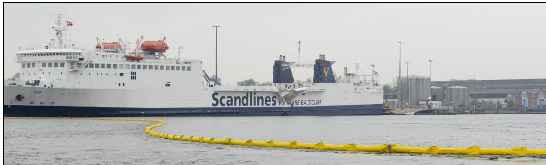
Figure 13: Deployed oil barrier
