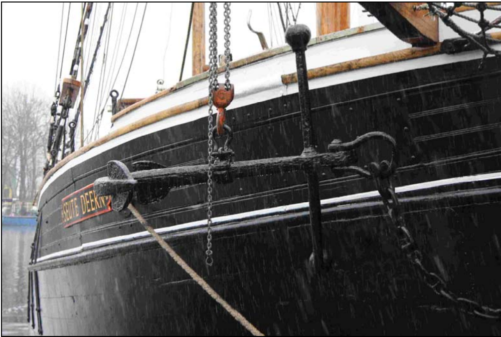
Figure 10: Stock anchor hoisted
