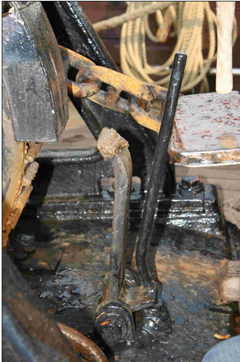
Figure 11: Pawl in tilt position
