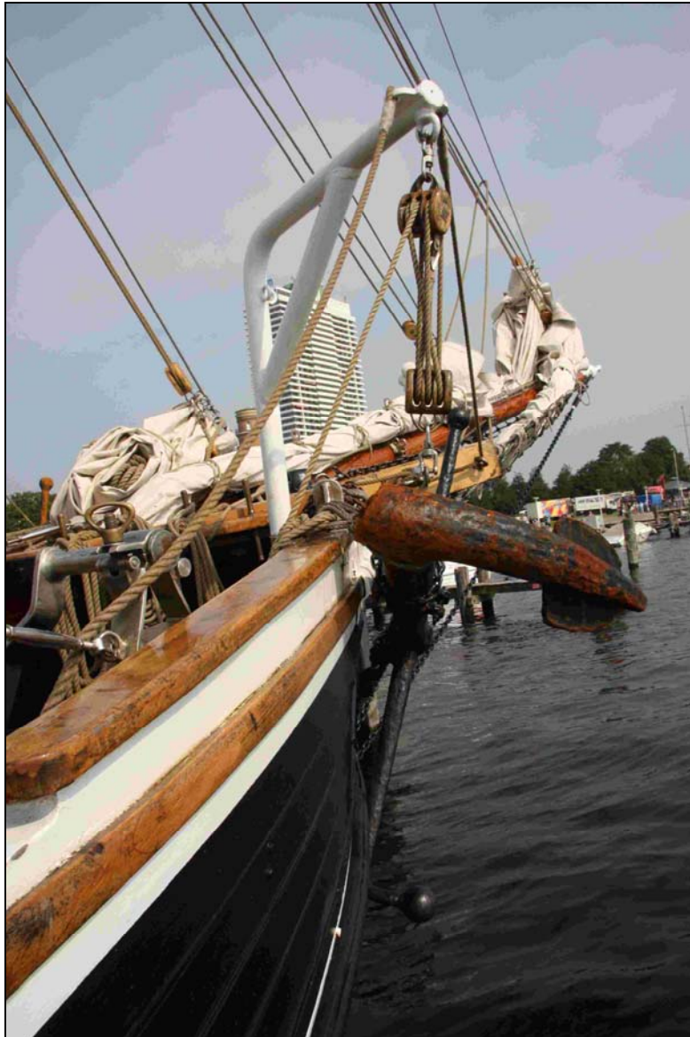
Figure 9: Stock anchor, missing fluke
