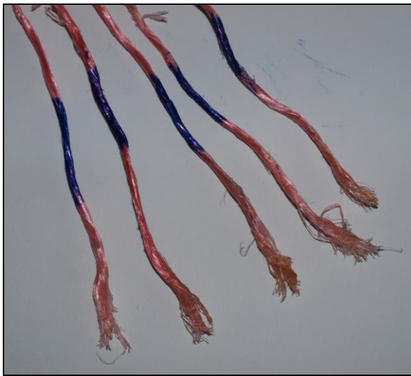
Figure 14: Damage before the break
