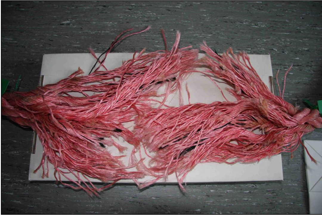
Figure 13: Point of failure on the stretcher
