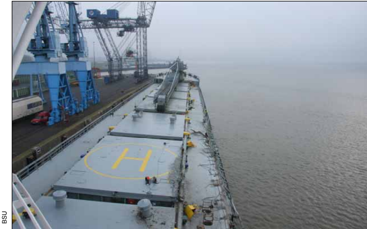
Figure 6: Destroyed starboard guard rail on SPLITTNES
