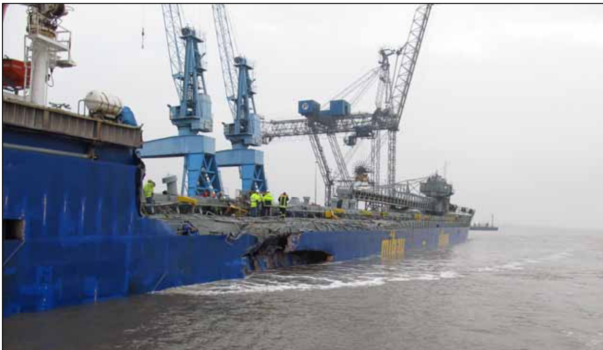
Figure 8: Water ingress on the starboard side of SPLITTNES
