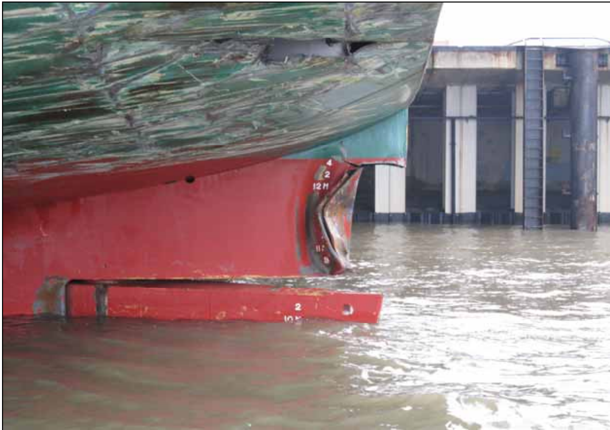
Figure 5: Damage to the rudder area of MOL EFFICIENCY
