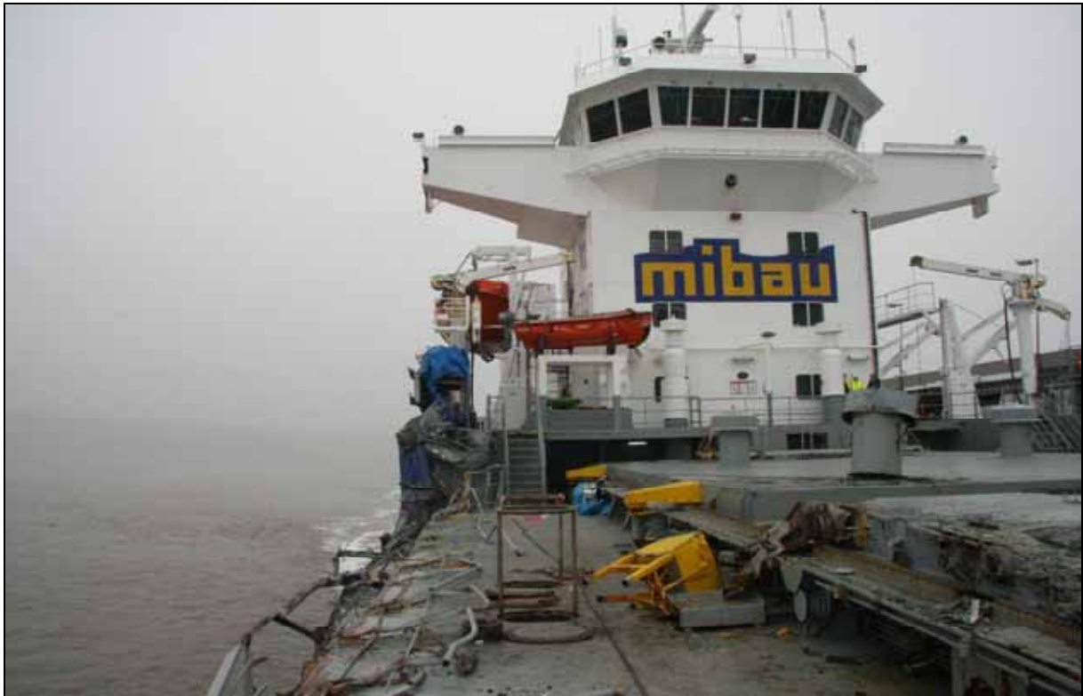
Figure 7: Destroyed main deck on SPLITTNES
