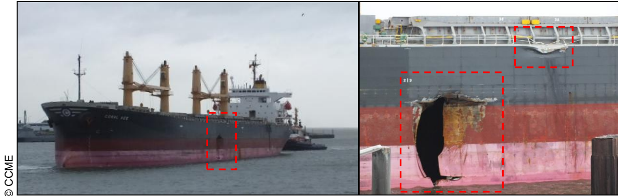
Figure 17: Damage on the port side of the CORAL ACE
