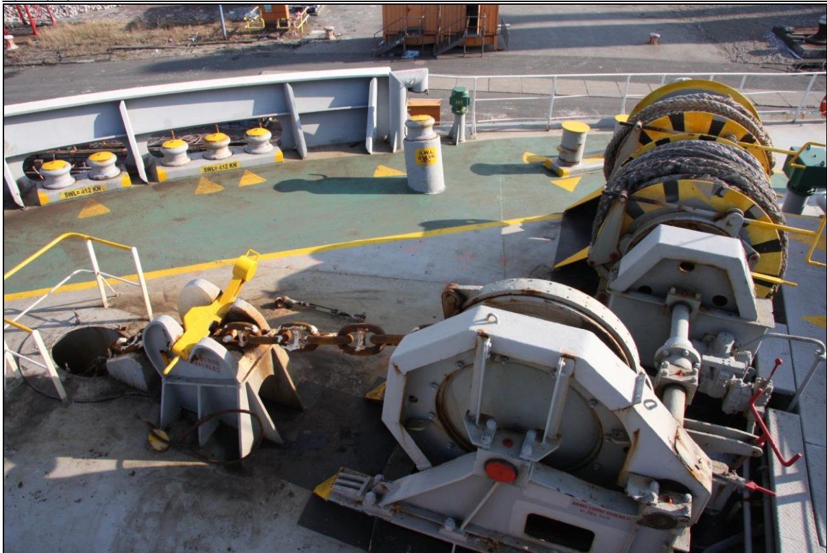
Figure 27: Starboard windlass and anchor chain on the fore section of the CORAL ACE
