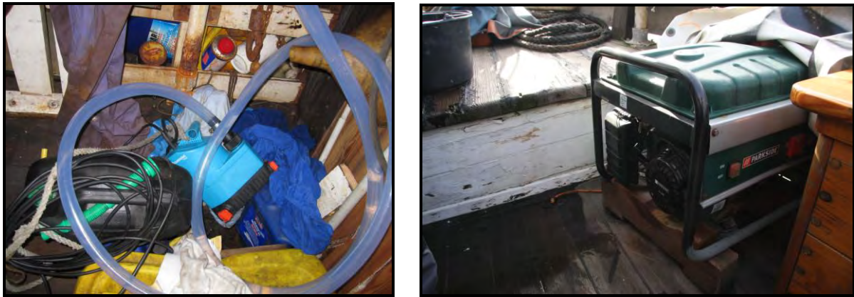
Figure 16: 220-volt garden pump and petrol-driven generator
