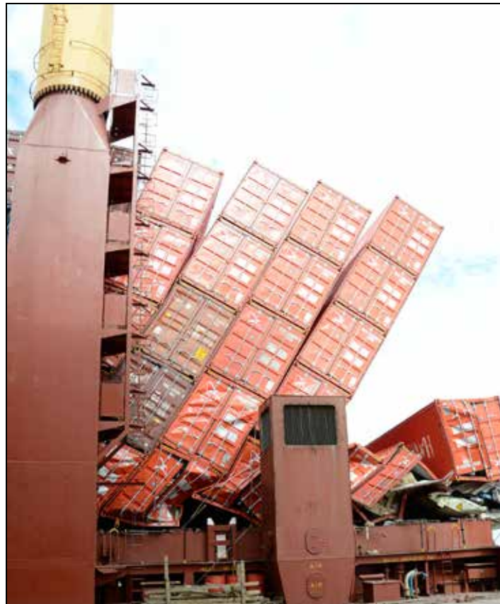
Figure 11: Tilted container stack (towards starboard) on the CCNI RIMAC 22
