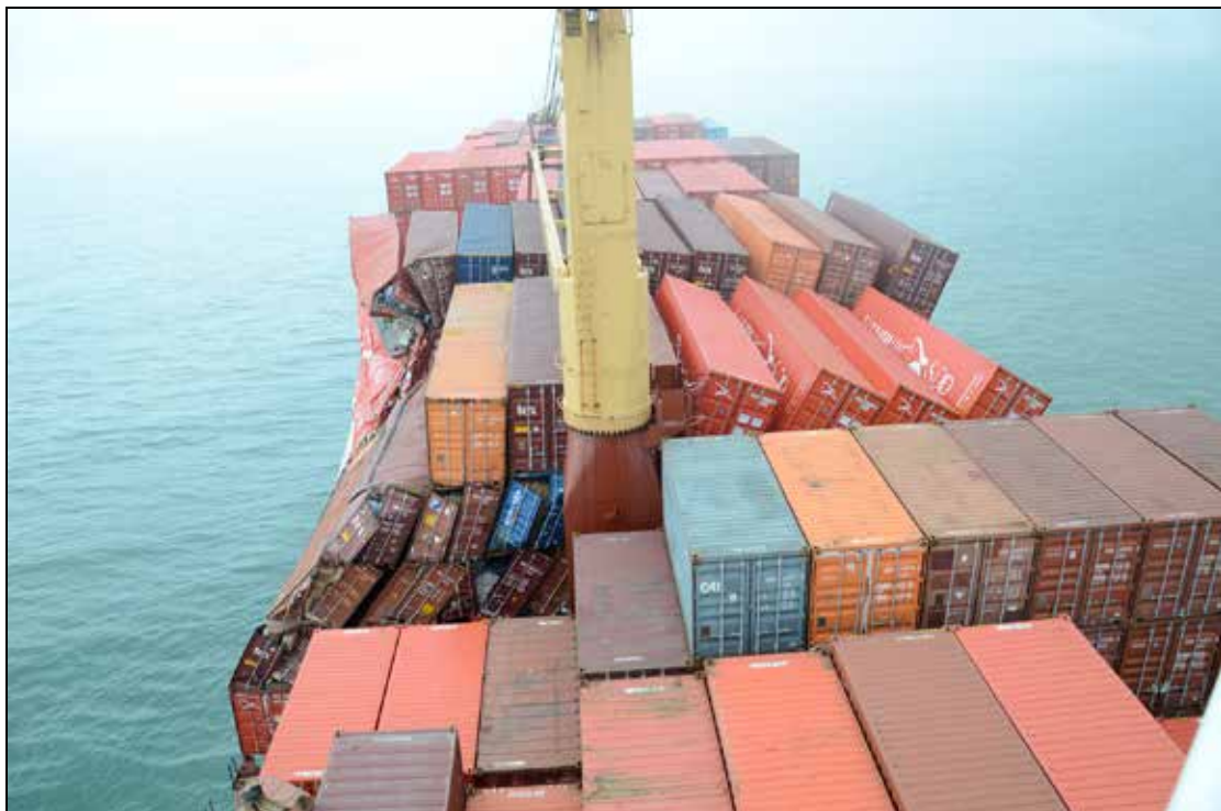
Figure 9: Damage to the deck cargo on the CCNI RIMAC (general view)
