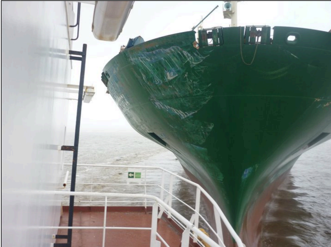
Figure 17: Paint abrasions on the bow of the CSAV PETORCA 23
