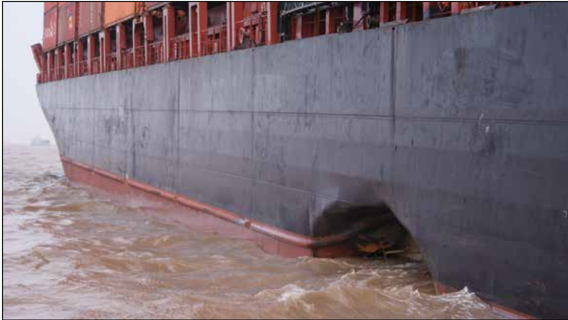
Figure 12: Damage to the shell plating on the CCNI RIMAC
