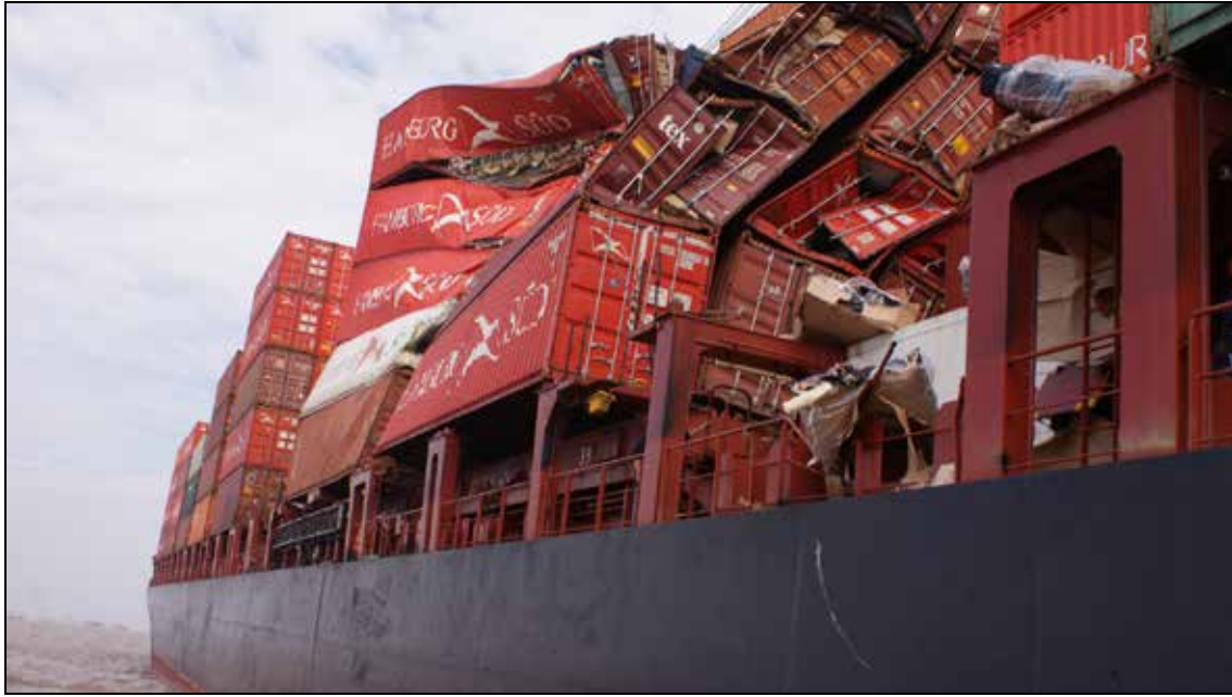
Figure 10: Damage to the deck cargo on the CCNI RIMAC (side view from port)
