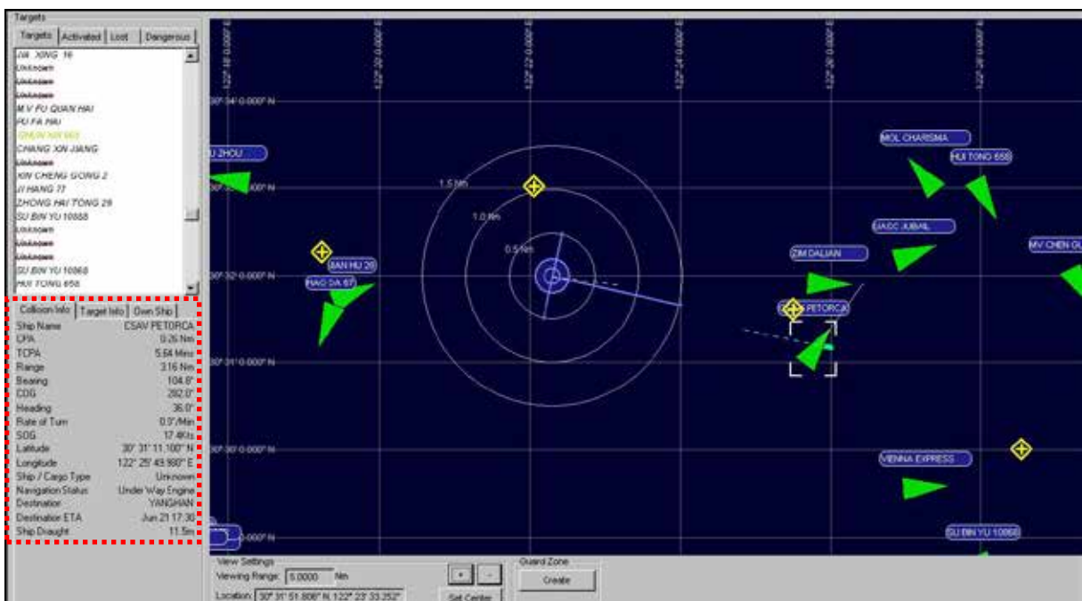
Figure 27: AIS display at 114703 (S-VDR replay)
