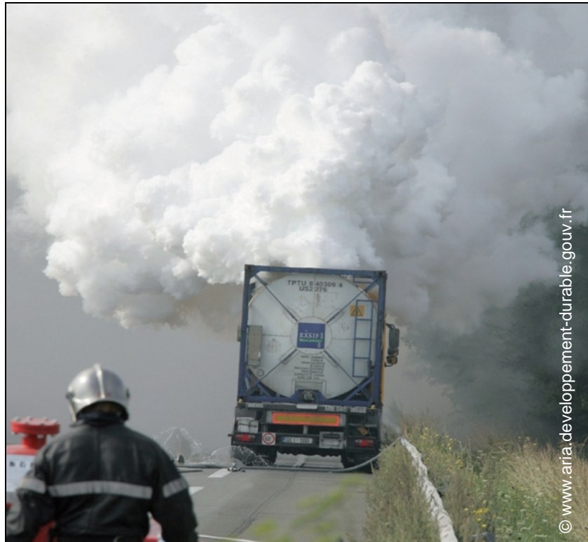
Figure 39: Ongoing polymerisation on a container in road transport
