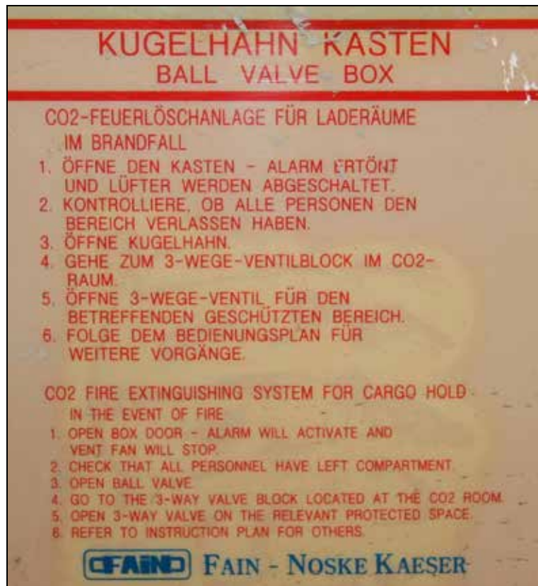
Figure 18: Description of the 'cargo hold' release procedure on the ball valve box
