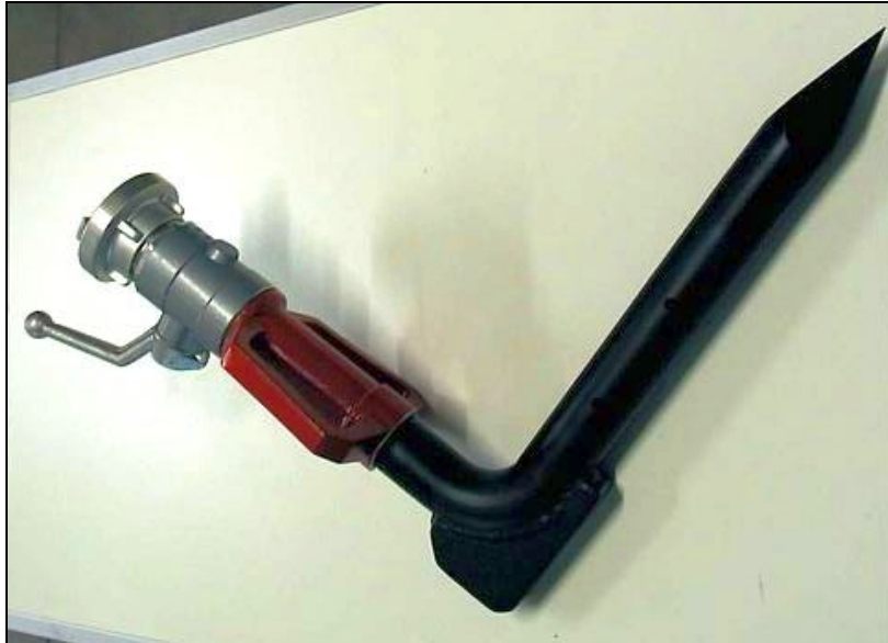
Figure 23: Fire-extinguishing lance for use on containers
