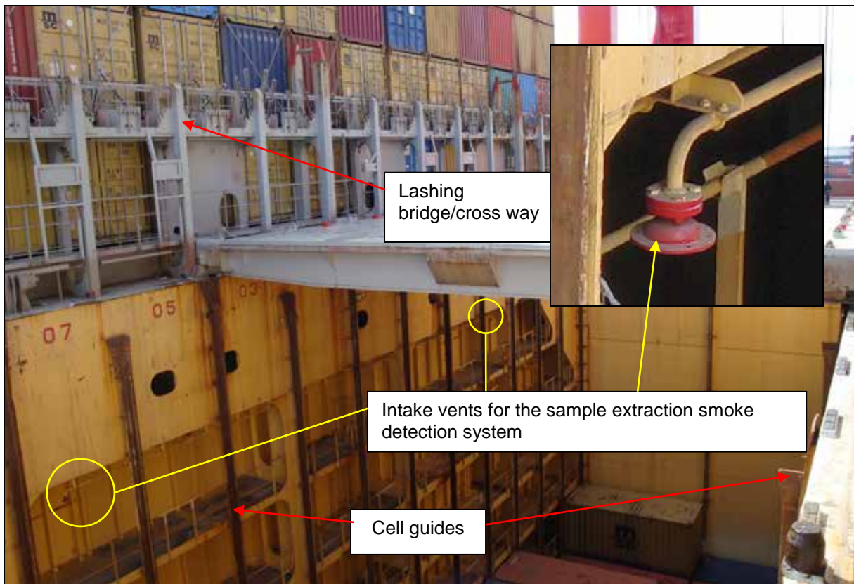
Figure 7: Sister ship (MSC ALESSIA). Aft edge of cargo hold 4, lashing bridge, middle hatch cover, improvement and intake vent for sample extraction smoke detection system
