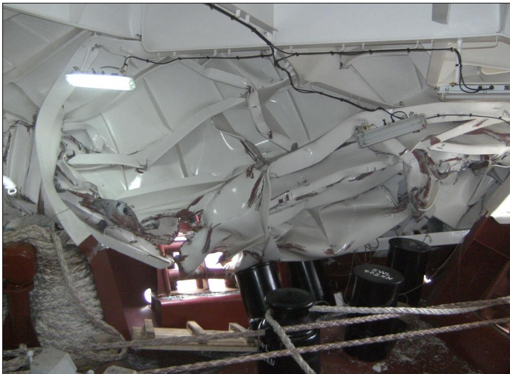
Figure 14: Damage to the forward manoeuvring station on the CMV CONMAR AVENUE
