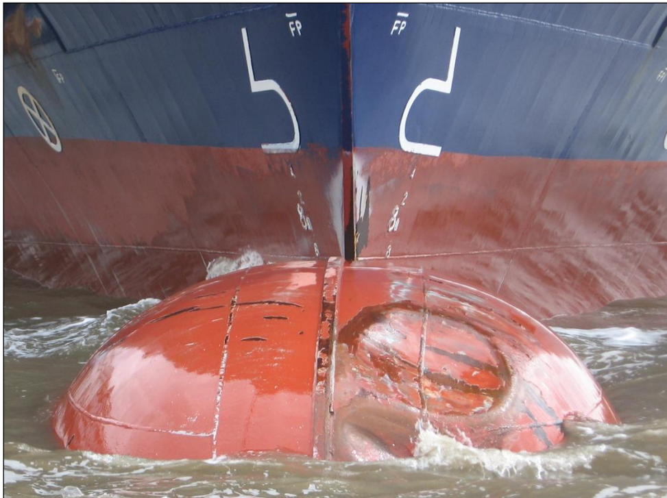
Figure 13: Deformed bulbous bow on the CMV CONMAR AVENUE
