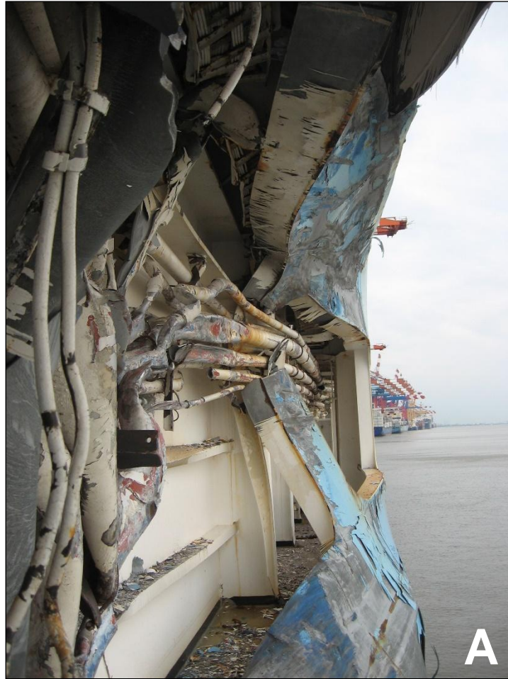
Figure 19: Damage to the hull wall – close-up (2)
