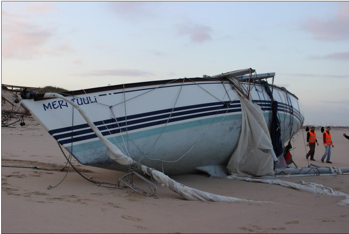
Fig. 25: Broken mast and railing
