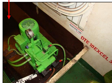
Figure 12: The hydraulic motor for the steering control is located on the floor below the switch cabinets
