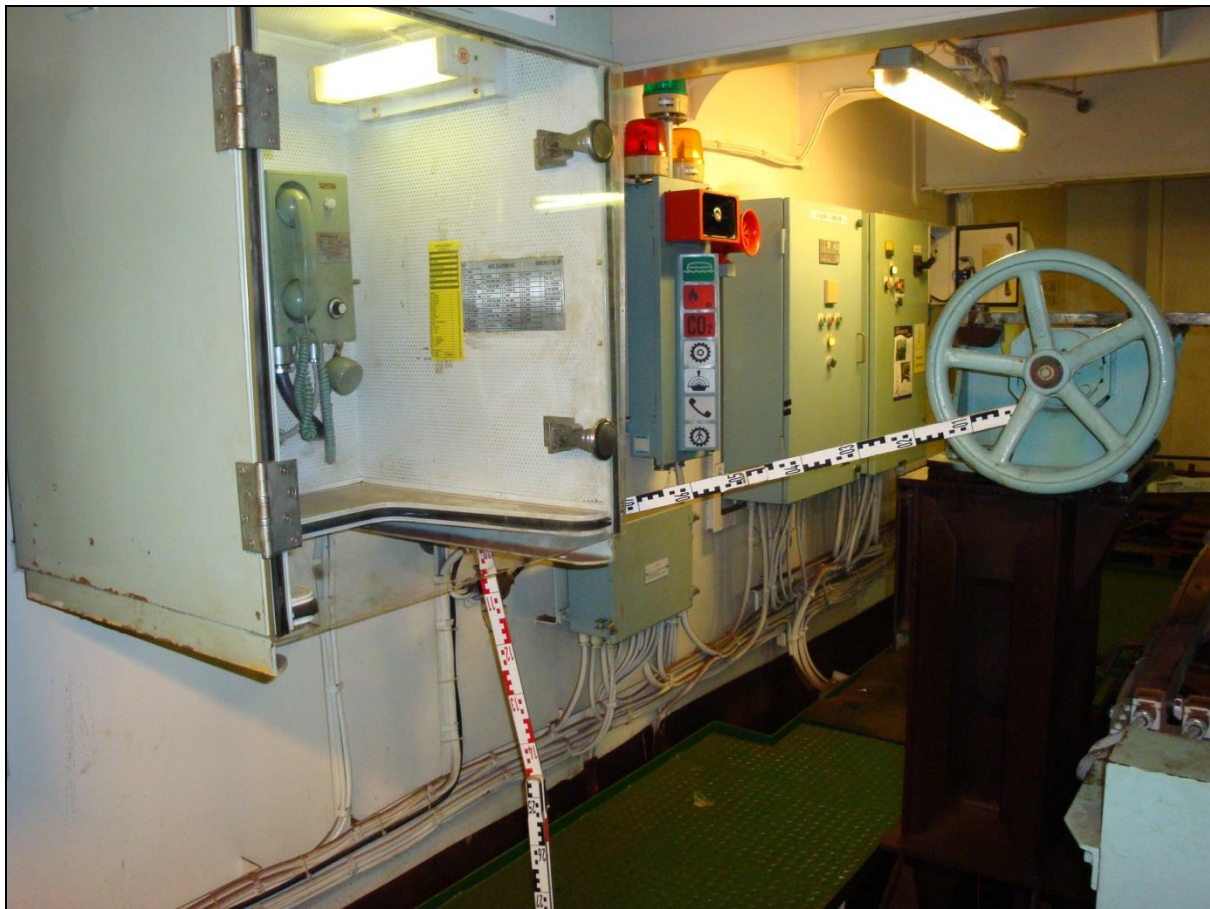
Figure 14: Distance from the phone to the hand wheel for operating the emergency rudder system
