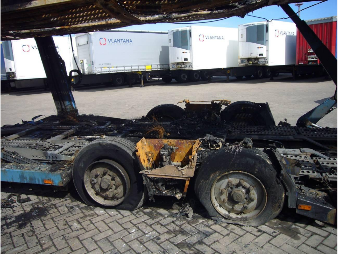
Figure 3: Burned down trailer
