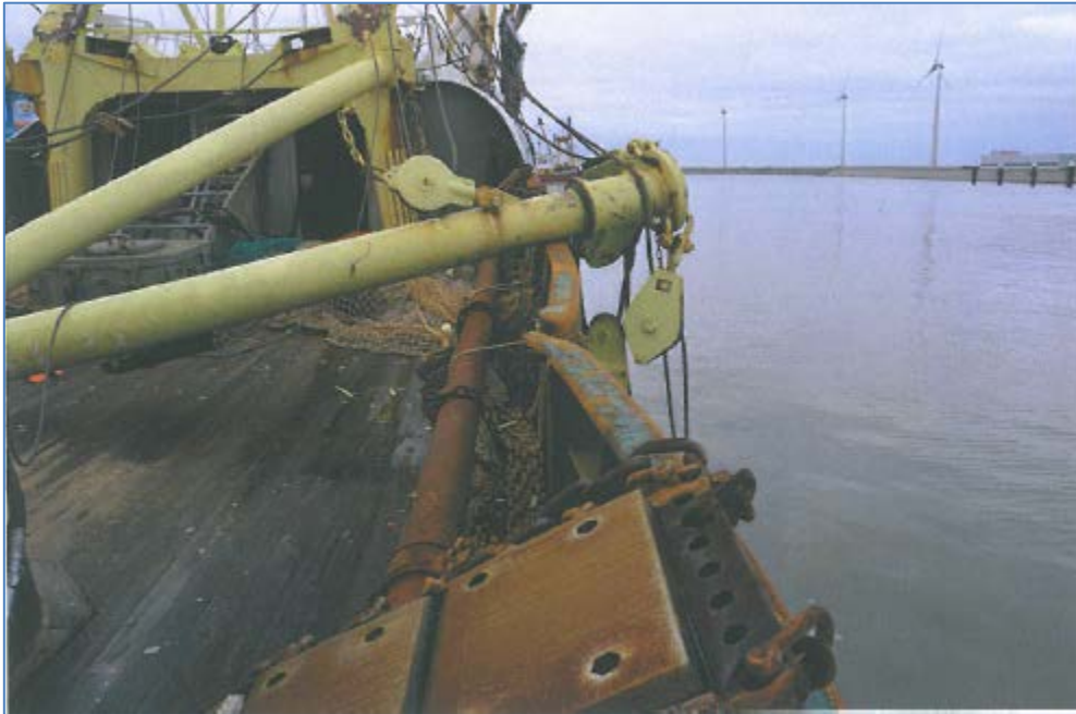
Figure 7: Damage to the starboard side and fishing gear
