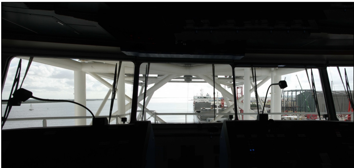
Figure 9: Obstructed visibility at the main steering position
