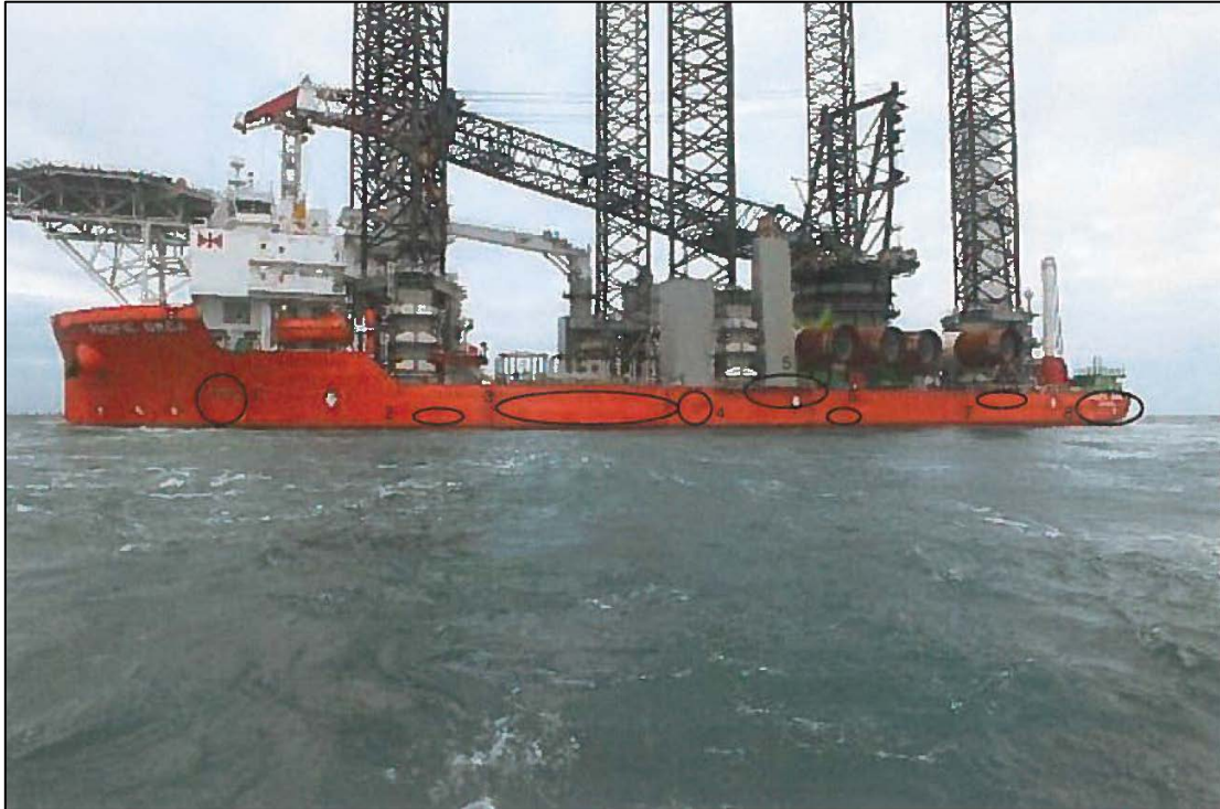
Figure 5: Apparent collision damage
