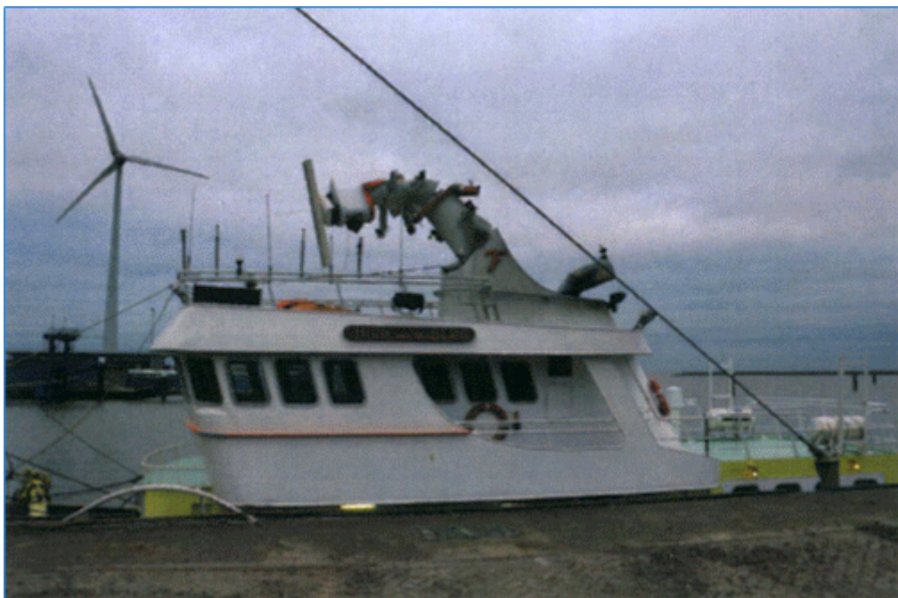
Figure 8: Buckled aft mast
