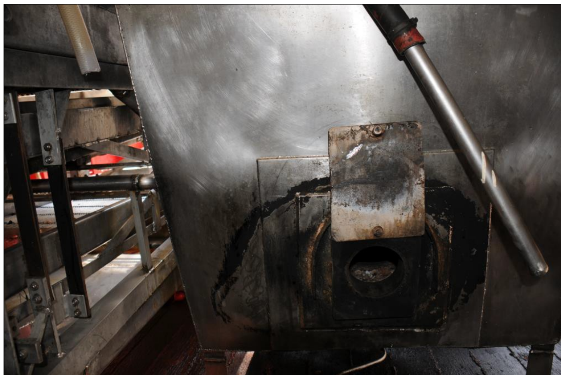
Figure 15: Fully open ignition aperture
