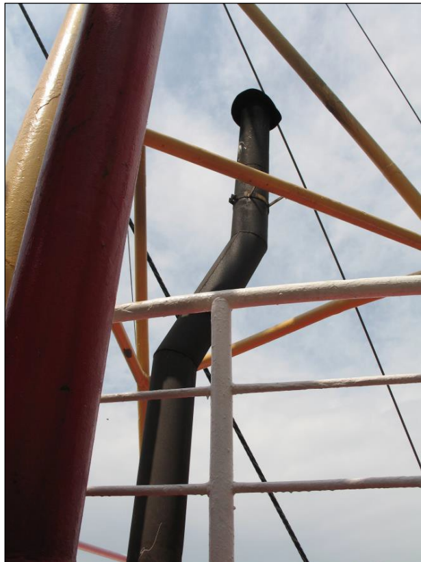
Figure 13: Exhaust pipe over the forecastle
