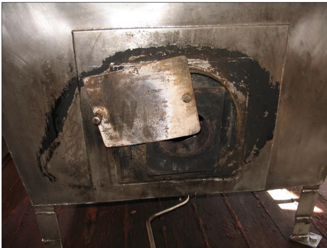
Figure 14: Ignition aperture with metal cover
