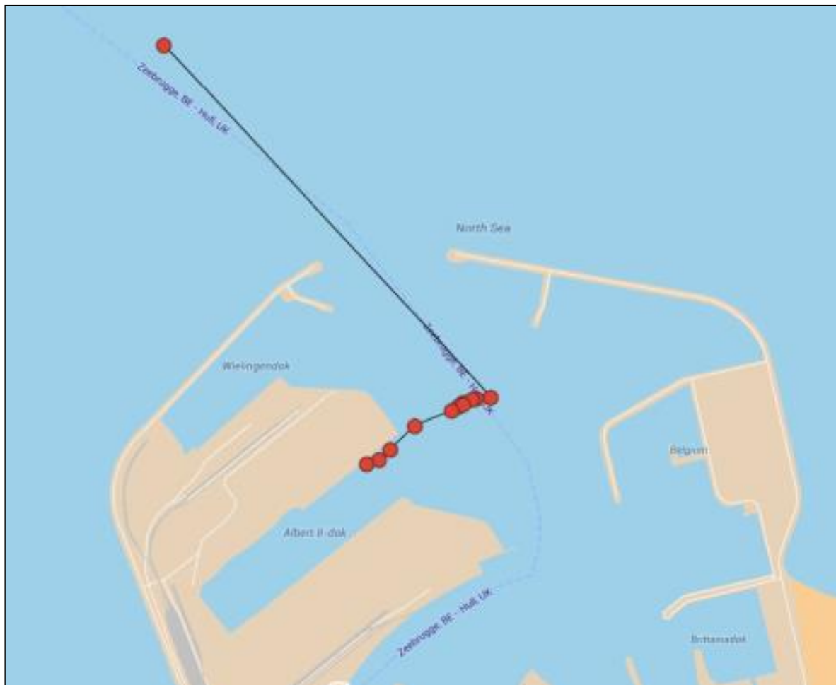
Figure 3: AIS track of the berthing manoeuvre
