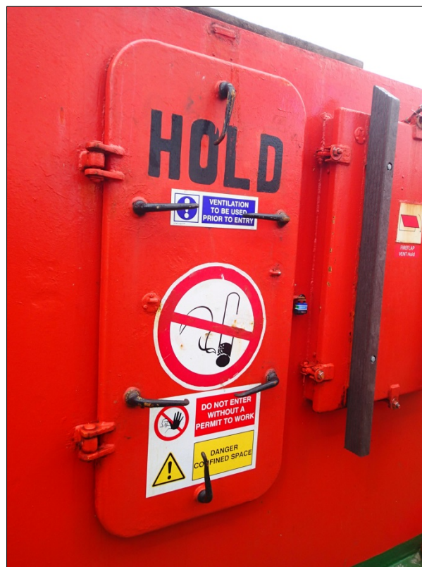
Figure 14: Cargo hold access and ventilation flap
