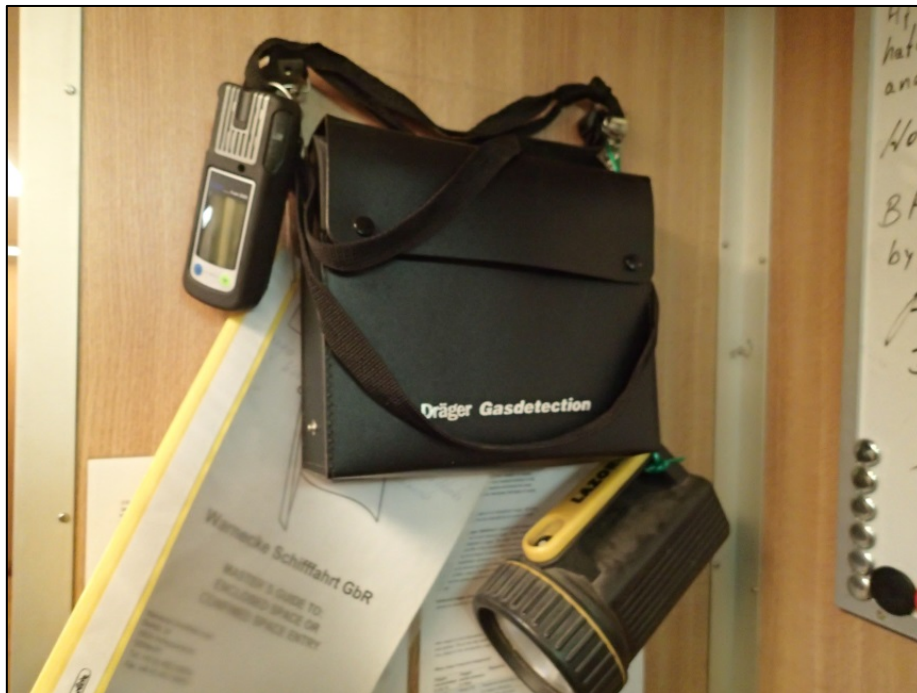
Figure 19: Gas monitors and data sheets
